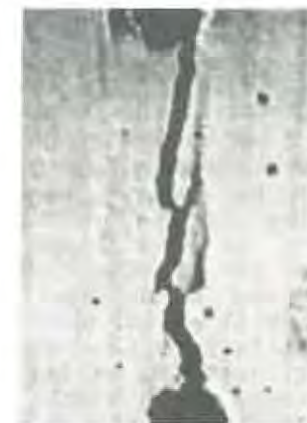
Figure 4. Double notch split cube ... fracture process
