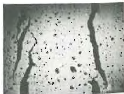
Figure 3. Fracture processes in badly compacted concrete with minimized friction at contact surfaces
