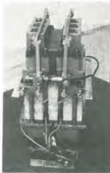
Figure 1. Test equipment showing the wedge of the splitting device, between the \sigma_1 -compressive load application structure with 4 screws (2 with strain gauges), one of the 2 LVDT's for COD recording.
