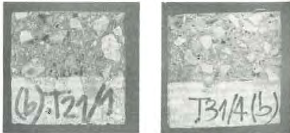
Figure 6. Typical fracture surfaces for fibre reinforced (left) and A2 (right) concretes.
