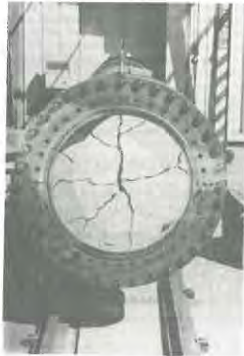
Figure 1. Cracked plain concrete slab at the end of the tube.
