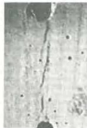
Figure 4. Double notch split cube ... fracture process
