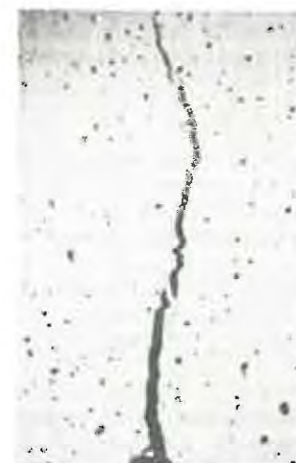
Figure 6. Crack development in 3-pt bending beam
