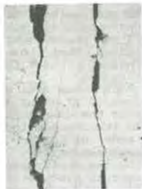
Figure 2. Formation of crack face bridges and compression struts in punch through shear specimen
