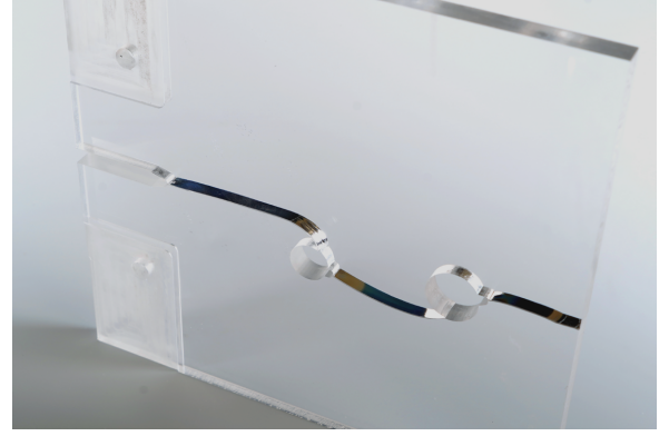
Figure 1: Fractured compact test specimen made of PMMA with an initial notch and 2 circular holes, each one having a tiny sharp notch [14].
