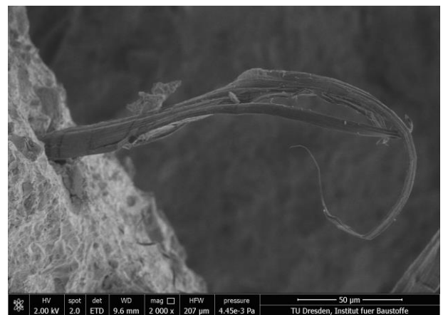
Figure 11. Ruptured fiber with an inclination angle of 30° in quasi-static loading regime
