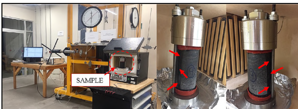
Fig.7 Set-up for high temperature tests in limestone samples. The arrows indicate the location of through cracks after the test at 100° C.
