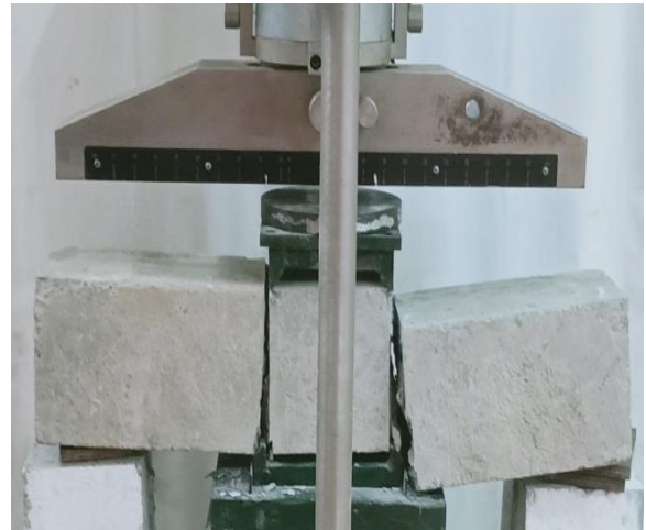
Figure 3: Failure of M30-0.50-Specimen No.3
