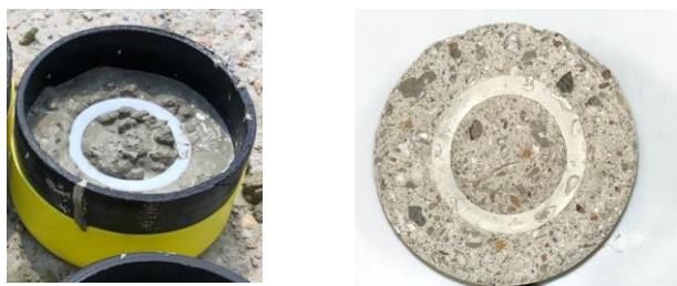
Figure 3: Placing the polymer insert (PTFE) during casting and broken half of a tested sample.
