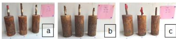
Fig 7. Typical cracked specimens a) 0.2 b) 0.50 c) 0.75 % of steel fibers in concrete
