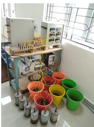
Fig 2. Test set up for accelerated corrosion
