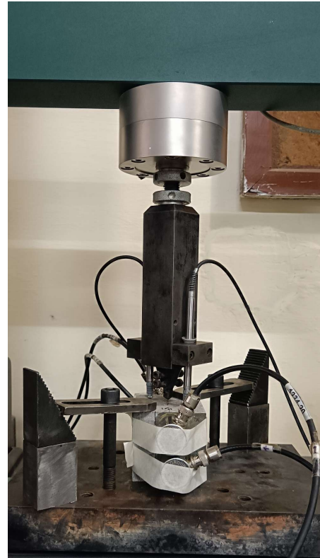
Figure 3: Fiber pullout and AE monitoring test.
