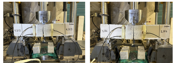
Figure 2: Test setup with beam containing 6 and 13 mm fibre.
