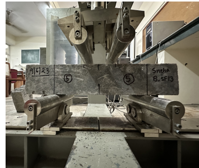
Figure 1: Four-point bend test specimen with 13 fibre length.
