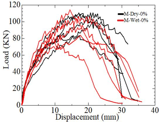
(a) Static pull-out tests
