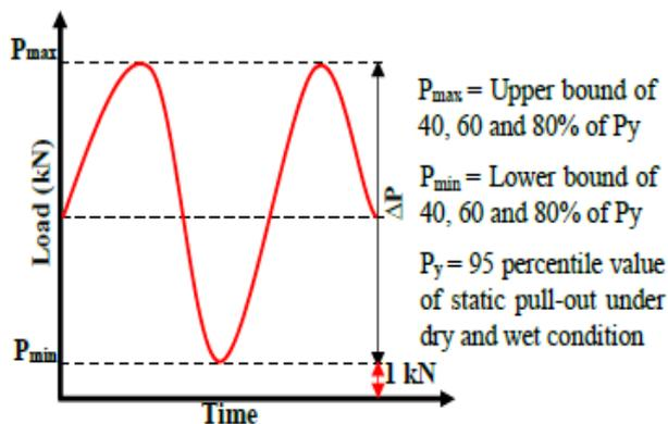
Figure 5: Conceptualized fatigue load (sine wave).
