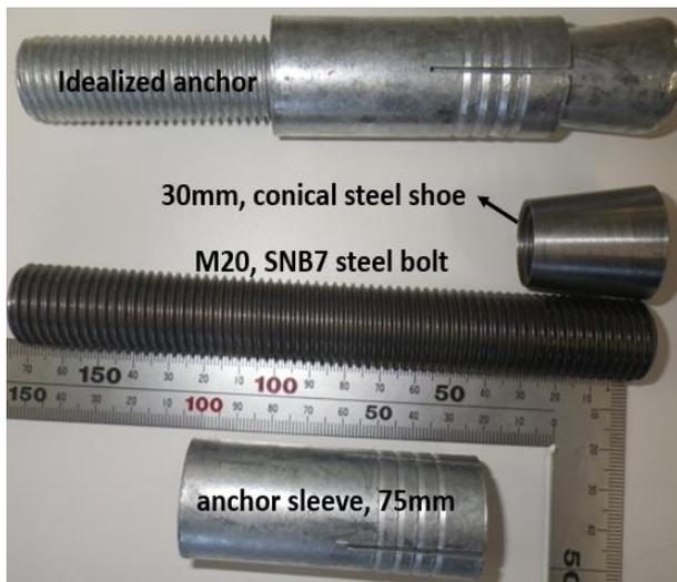
Figure 2: Modified anchor using high strength bolt.
