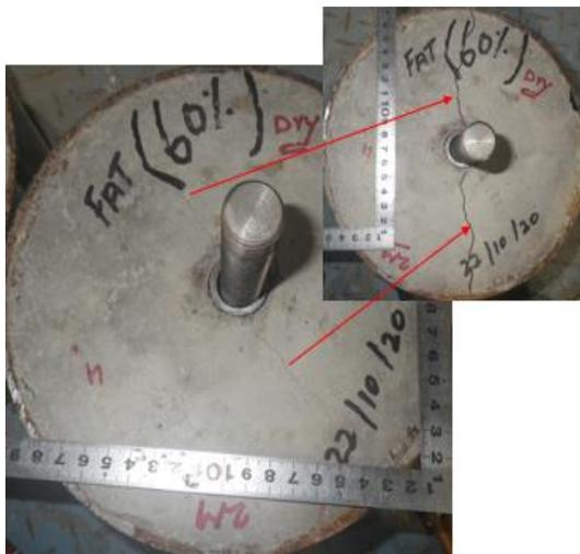
**Figure 9:** Concrete fatigue crack.
