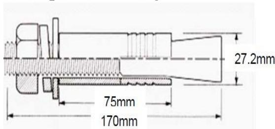
Figure 1: Details of used anchor.
