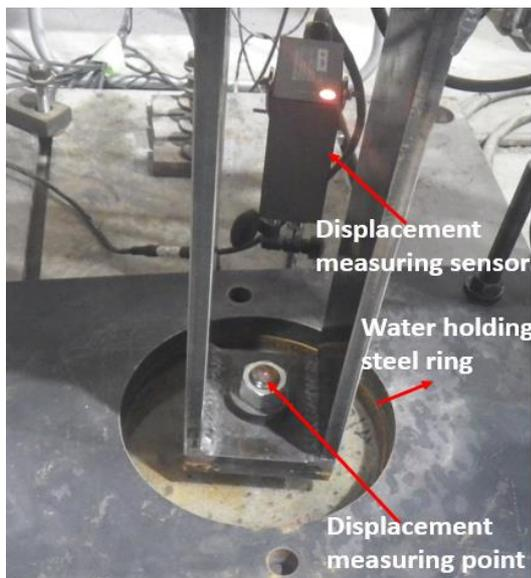
Figure 4: Fatigue test in wet condition.
