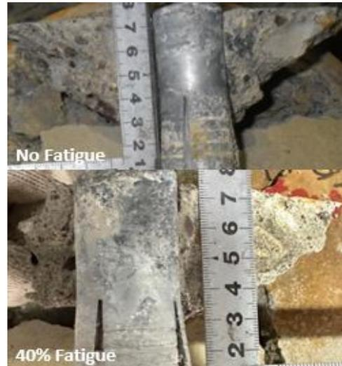
**Figure 12:** Concrete cone failure before and after fatigue loading.
