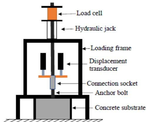
Figure 6: Pull-out test setup.
