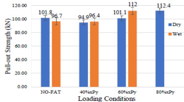
**Figure 10:** Residual pull-out strength.
