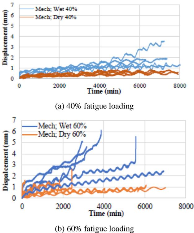
**Figure 8:** Pull-out displacement under 40% and 60% loading.
