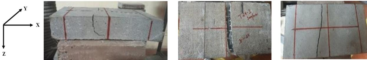
Figure 15: Crack propagation and failure pattern of specimens
