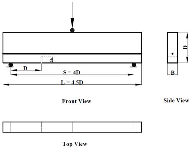
**Figure 1:** Details of geometry of the specimens
