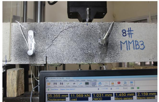
Figure 13: Failure pattern for medium size with 8mm bar (0.67 %)
