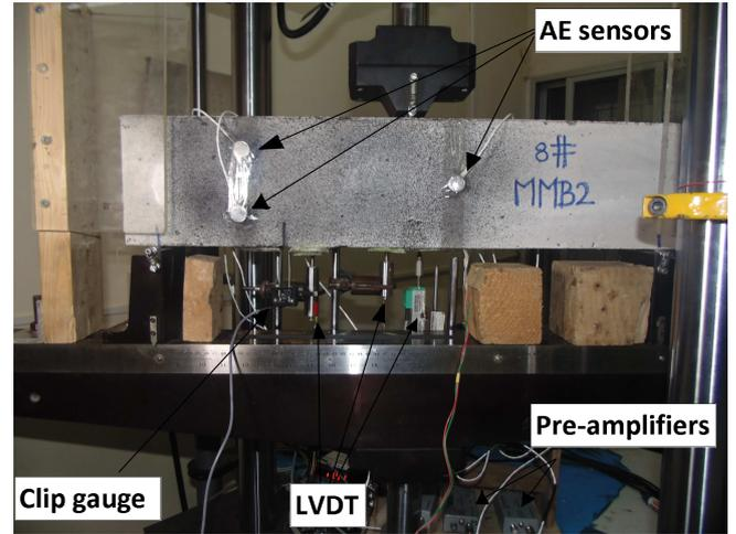
**Figure 2:** Testing of beam specimen and instrumentation such as clip gauge and LVDT and strain gauge to reinforcement
