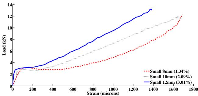
Figure 5: Load versus Strain for small size specimens with different percentage variation of reinforcement
