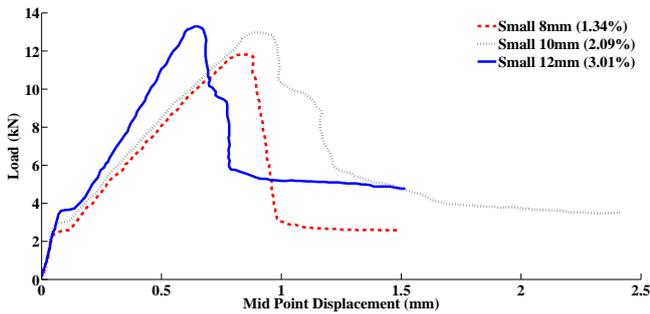
Figure 4: Load versus Mid Point Displacement for small size specimens with different percentage variation of reinforcement
