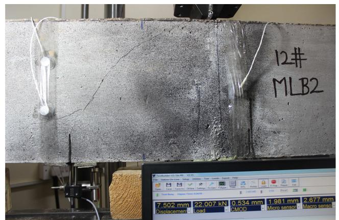
Figure 14: Failure pattern for large size with 12mm bar (0.75 %)
