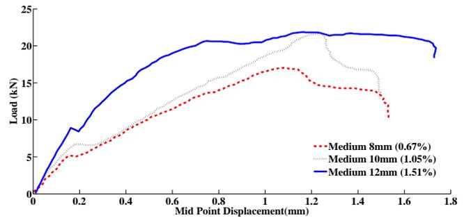
Figure 7: Load versus Mid Point Displacement for medium size specimens with different percentage variation of reinforcement
