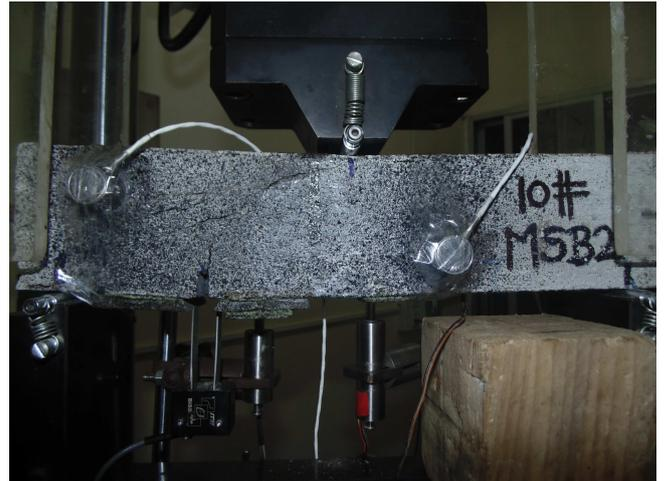
Figure 12: Failure pattern for small size with 10mm bar (2.09 %)
