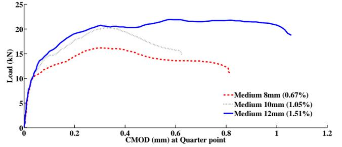
Figure 6: Load versus CMOD at Quarter Point for medium size specimens with different percentage variation of reinforcement
