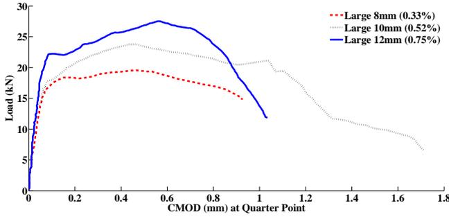
Figure 9: Load versus CMOD at Quarter Point for large size specimens with different percentage variation of reinforcement
