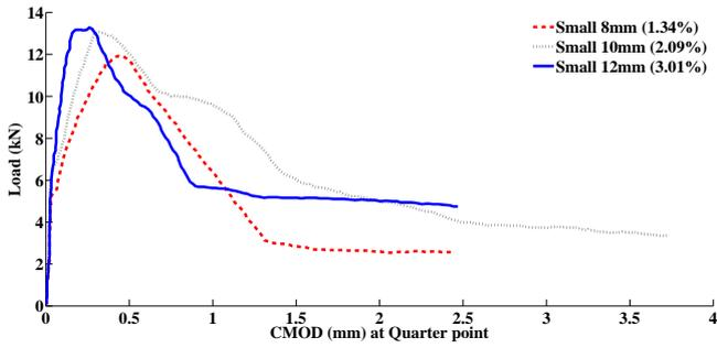
Figure 3: Load versus CMOD at Quarter Point for small size specimens with different percentage variation of reinforcement
