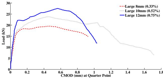
Figure 10: Load versus Mid Point Displacement for large size specimens with different percentage variation of reinforcement
