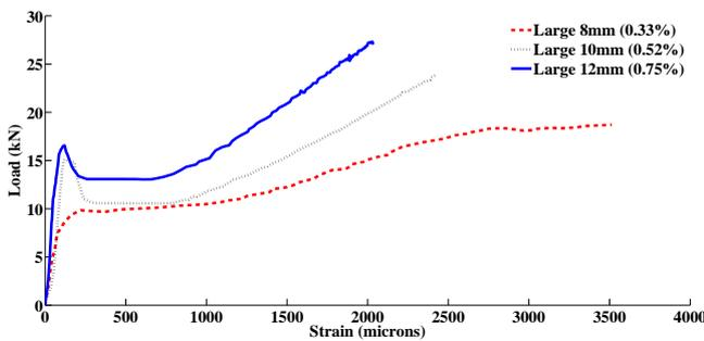
Figure 11: Load versus Strain for large size specimens with different percentage variation of reinforcement
