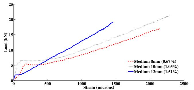
Figure 8: Load versus Strain for medium size specimens with different percentage variation of reinforcement
