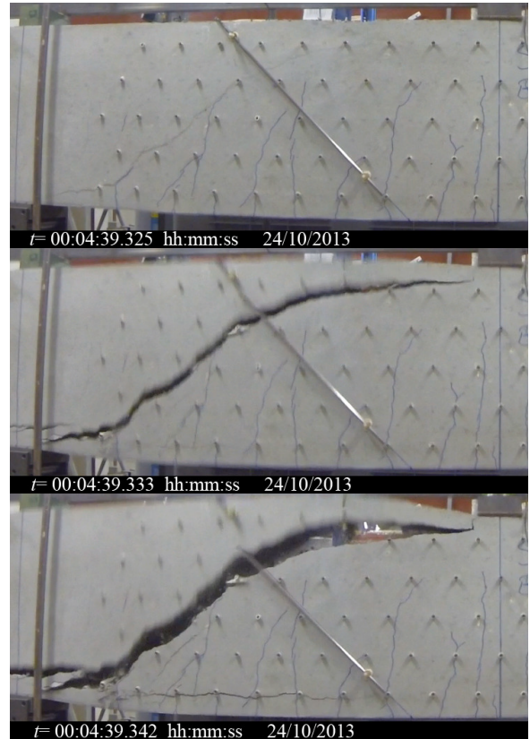
Figure 12: Shear critical RC beam within \Delta t = 0.01 s, taken from [12].
