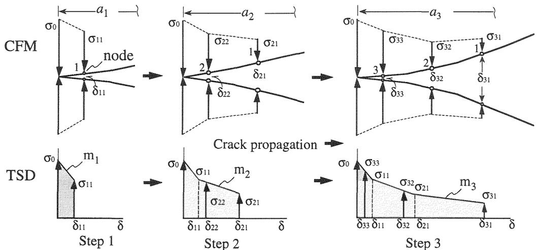
Fig. 3. Concept of poly-linear approximation analysis of TSD
