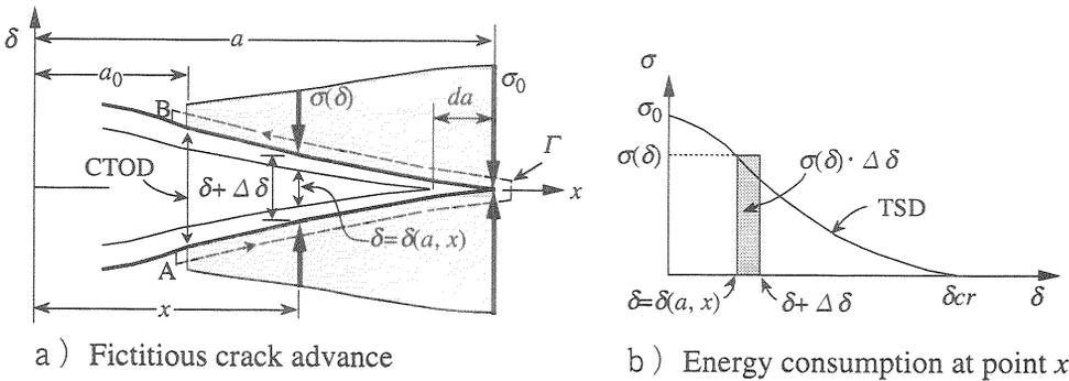
Fig. 4. Fictitious crack advance and energy consumption
