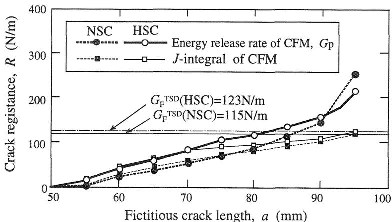
Fig. 10.  $R$ -curve of cohesive force model (CFM)
