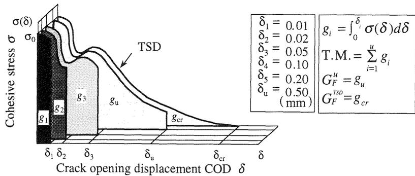
Fig. 11. Fracture toughness parameters based on poly-linear TSD
