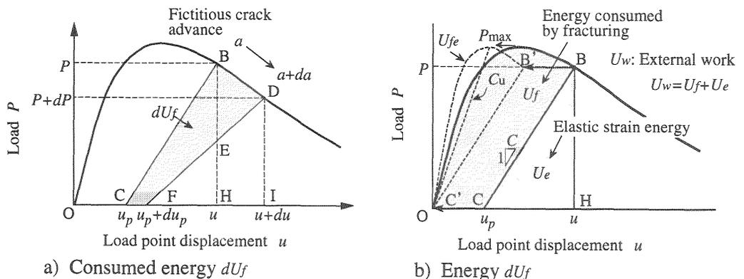
Fig. 5. Relation of L-LPD curve and energy consumption
