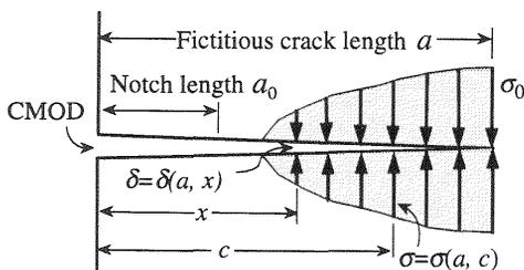
Fig. 1. Cohesive force model(CFM)
