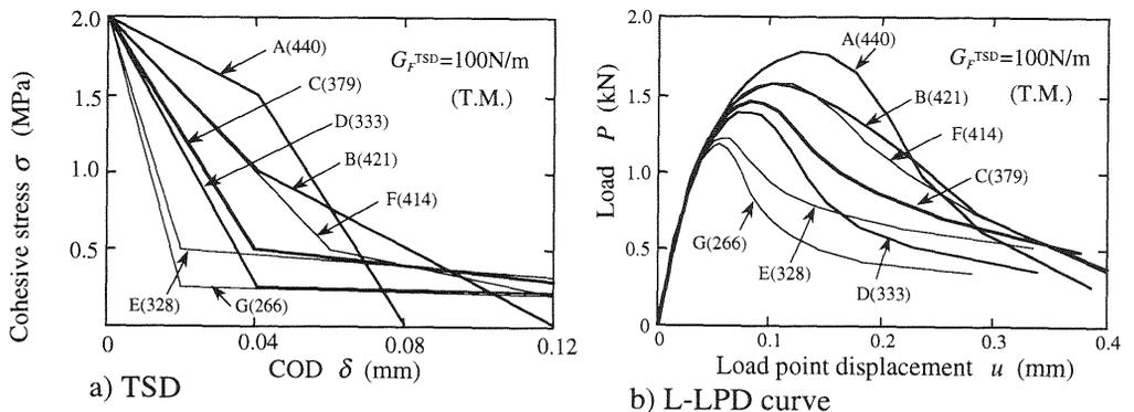
Fig. 12. Relation of T.M. and L-LPD curve with same fracture energy of TSI
