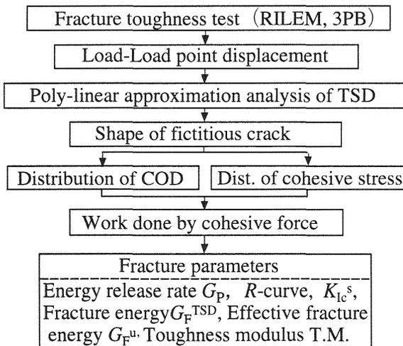
Fig. 7. Analysis flow of fracture parameters
