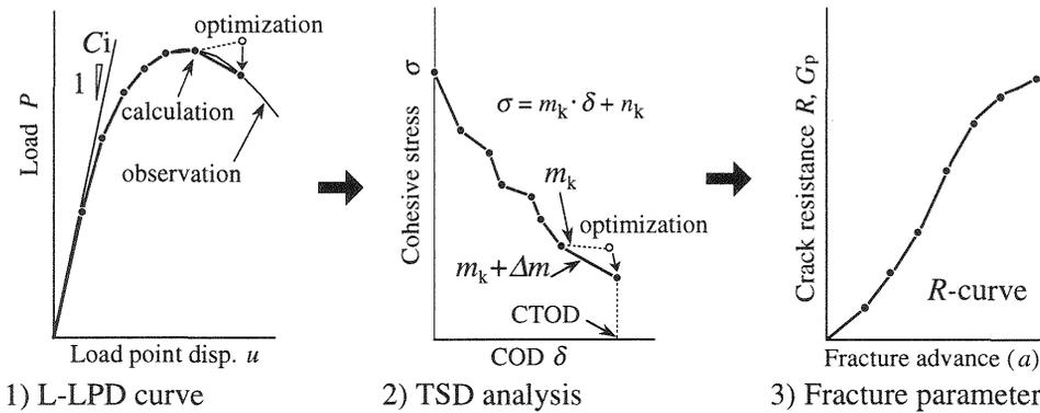
Fig. 6. Procedure of fracture parameter analysis
