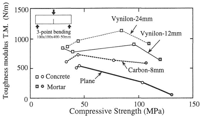
Fig. 13. Toughness modulus(T.M.) and compressive Strength
