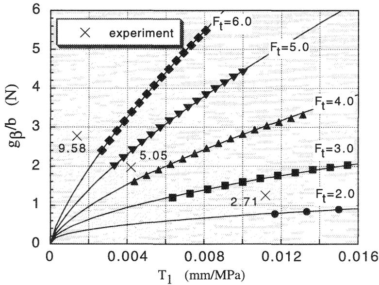
Fig. 7.  $g\beta/b$ - $T_1$  relationship for wedge splitting test
