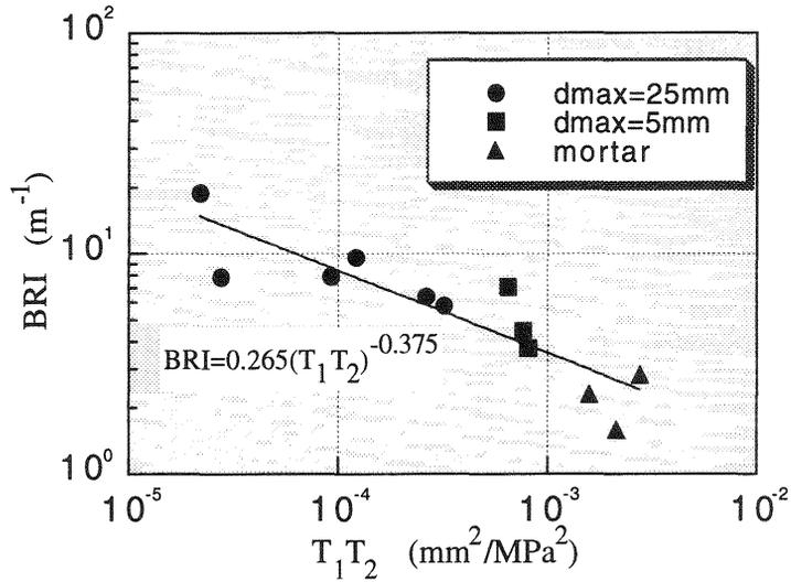
Fig. 8. Relation between brittleness parameters
