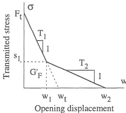
Fig. 1. Parameters notation in bi-linear tension softening model
