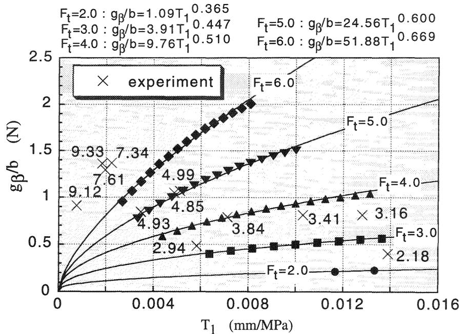
Fig. 6.  $g_\beta/b-T_1$  relationship for three point bending test
