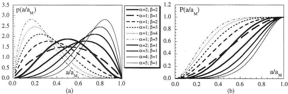
Fig. 3. Truncated defect size distribution by varying the parameters  $\alpha$  and  $\beta$ :
