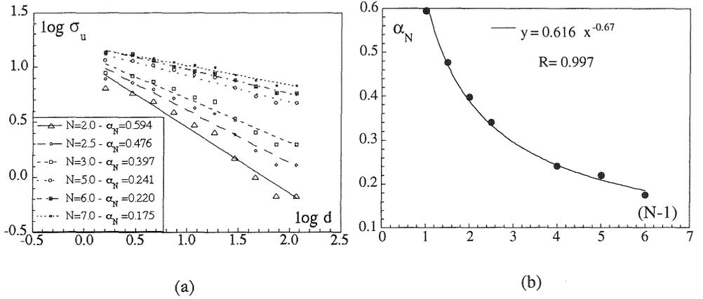
Fig. 2. (a) Strength size effect laws for a tridimensional body by varying the statistical dispersion parameter  $N$  ( $a_0=1\text{mm}$ ). (b) Power law that relates the slope  $\alpha_N$  of the straight line with the parameter  $N$ .
