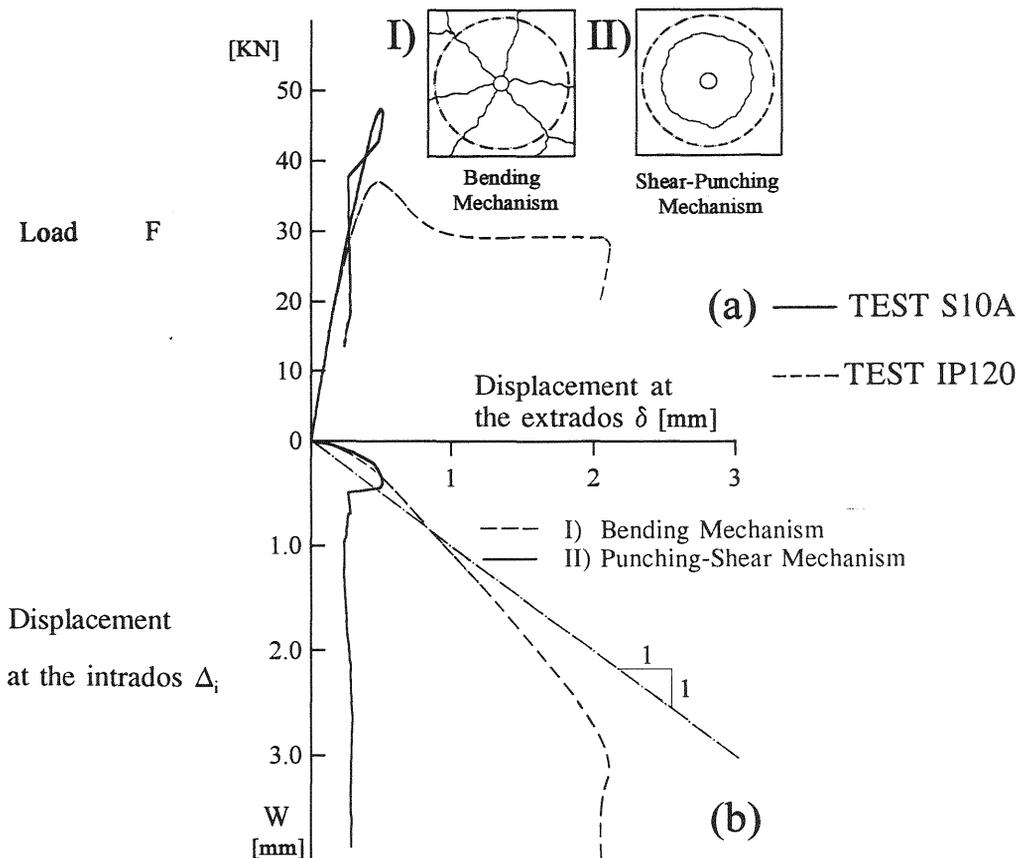
Fig. 9 - Typical load-displacement and displacement-displacement curves for punching failures characterized mostly by bending (I) and by shear (II): (a) load versus displacement at the extrados  $\delta$ , and (b) displacement at the intrados  $\Delta_i$  versus displacement at the extrados. PAN fibers,  $v_f = 1\%$ ,  $\lambda = 600$  in test S10A,  $\lambda = 120$  in test IP120.
