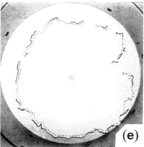
Fig. 10 - Typical evolution of crack pattern in static tests: (a) load-displacement curve of Test P15B (PAN fibers, fiber content 1.5% by volume,  $l_f = 12$  mm,  $d_f = 100 \mu\text{m}$ ); (b) bending cracks; (c) bending and shear cracks; (d, e) shear cracks.  $P_{\max} = 53.1$  kN.
