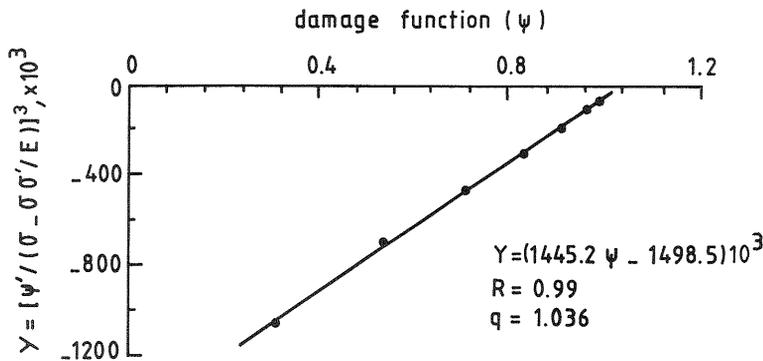
Fig.6. Y versus damage function relationship evaluated from the test results given by Taşdemir (1982)
