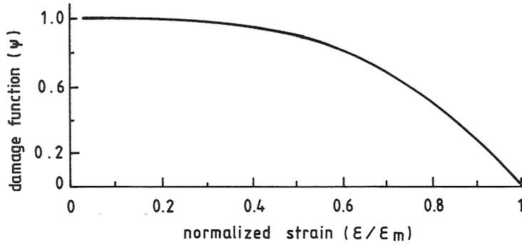
Fig.5. The variation of damage function with respect to  $\epsilon/\epsilon_m$
