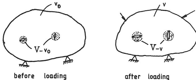
Fig.2. A solid body with flaws before and after loading
