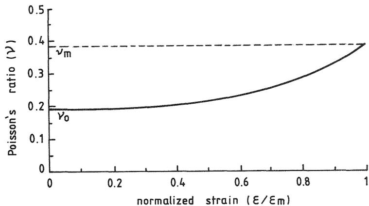
Fig.4. Poisson's ratio versus normalized strain curve
