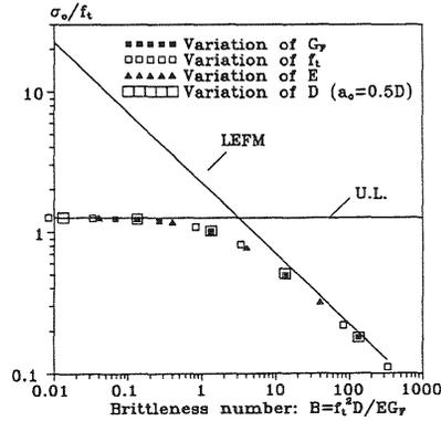
Fig. 3. Failure load versus Brittleness Number
