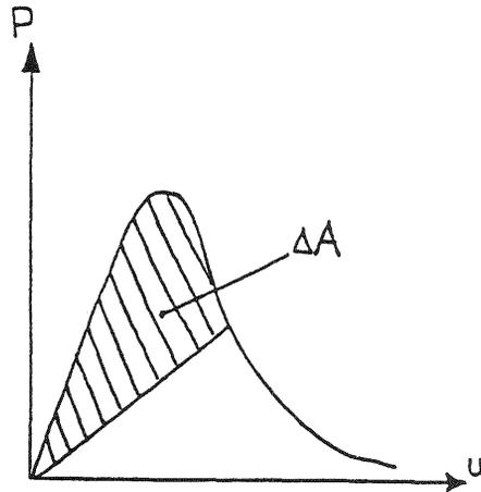
Fig. 2. Definition of the area  $\Delta A$  from the load-deflection curve
