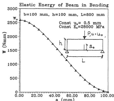
Fig. 1. Elastic energy  $W$  for three point bending under constant displacement
