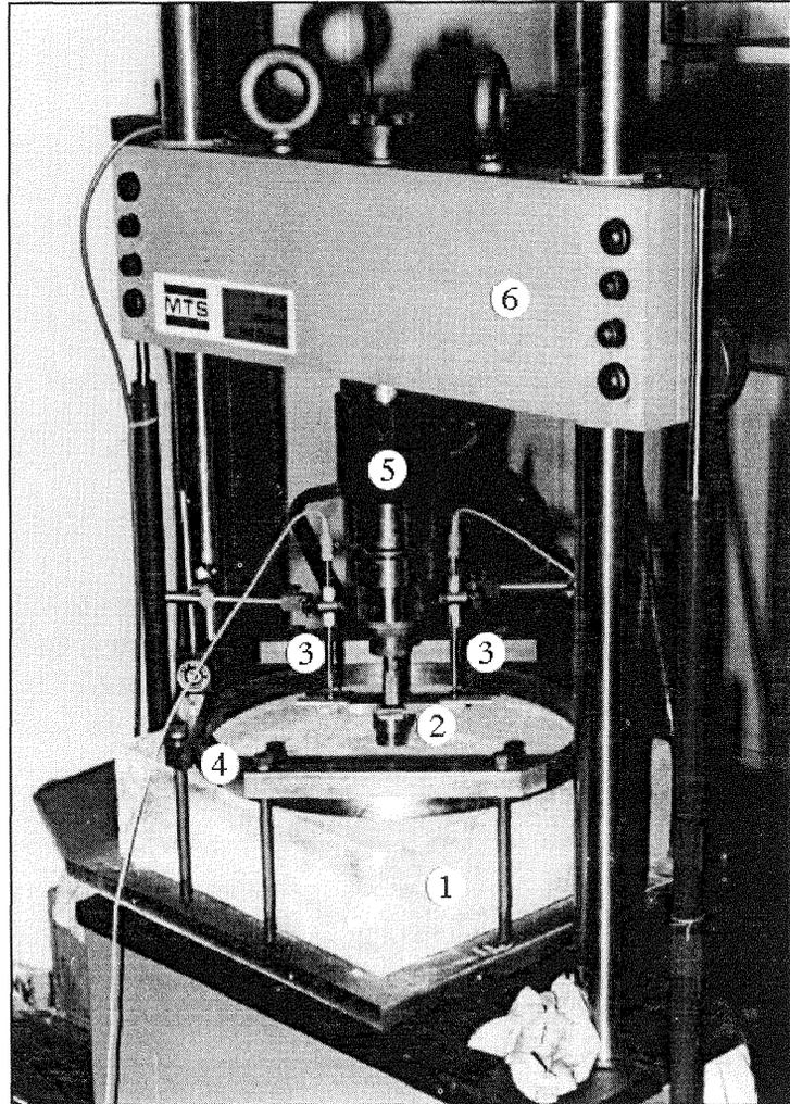
Fig. 1. Layout of testing equipment: 1. Specimen; 2. Extractor; 3. LVDT; 4. Contrast ring; 5. Load cell; 6. MTS
