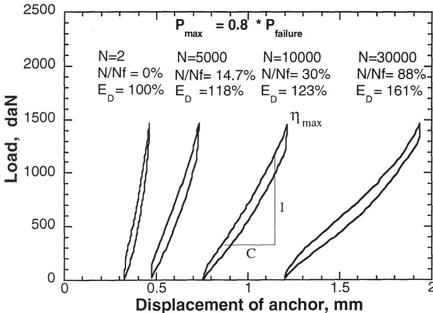
Fig. 3. Variation of cycle shape in fatigue test.
