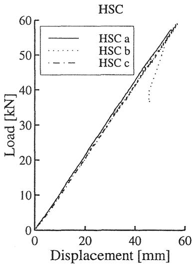
Fig. 4. Load displacement curves for HSC.
