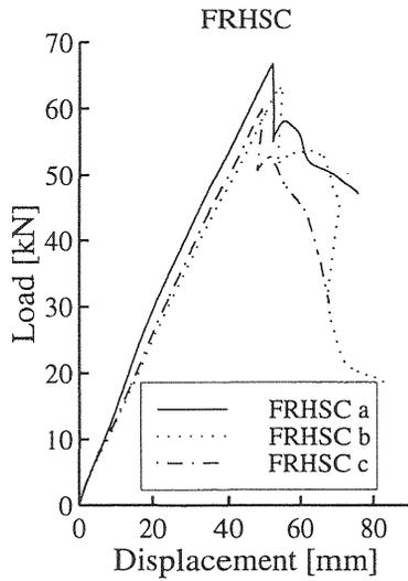
Fig. 6. Load displacement curves for FRHSC.
