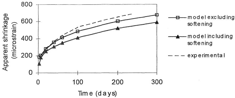
Fig. 6. Shrinkage for small specimen (75 x 50 x 250)
