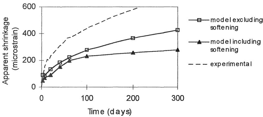
Fig. 7. Shrinkage for medium-sized specimen (150 x 100 x 500)
