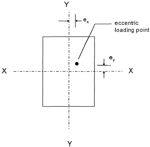
Several sets of creep measurements were obtained using medium and large specimens with various loads and load eccentricities as shown in Table 1.
