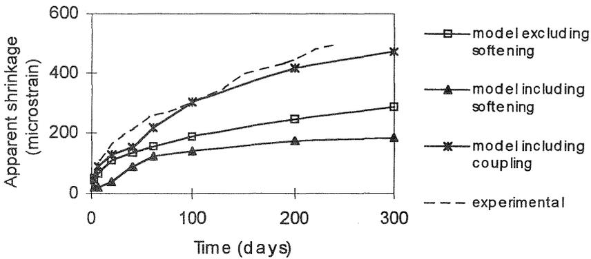
Fig. 8. Shrinkage for large specimen (300 x 200 x 1,000)
