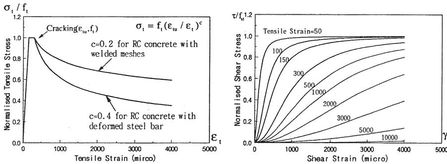
Fig. 2. Tension and shear stiffening model for concrete in RC zone
