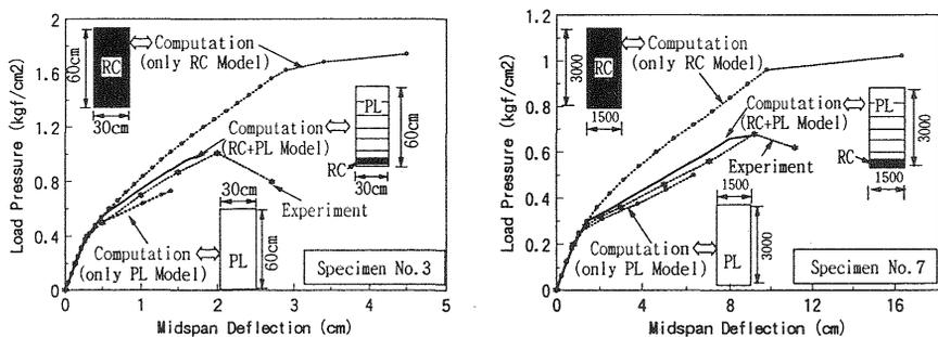
Fig. 7. Load-deflection relation for different specimen at midspan
