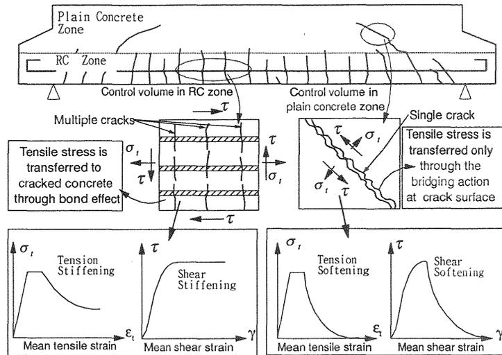
Fig. 1. The different models of cracked concrete in RC structure
