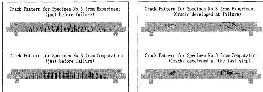
Fig. 9. Crack patterns for specimen No.3
