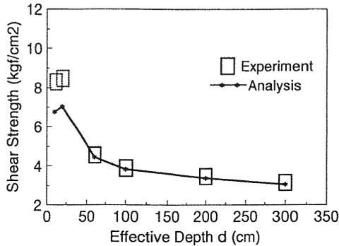
Fig. 8. Shear strength and effective depth
