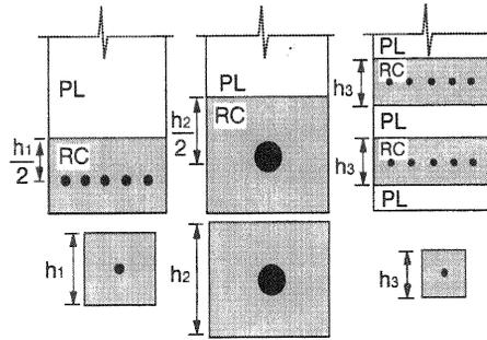
Fig. 4. RC zone definition in computation
