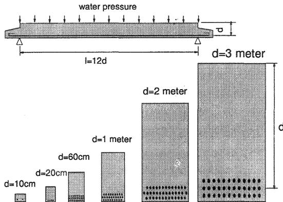
Fig. 6. Details of cross sections and arrangement of reinforcing bars
