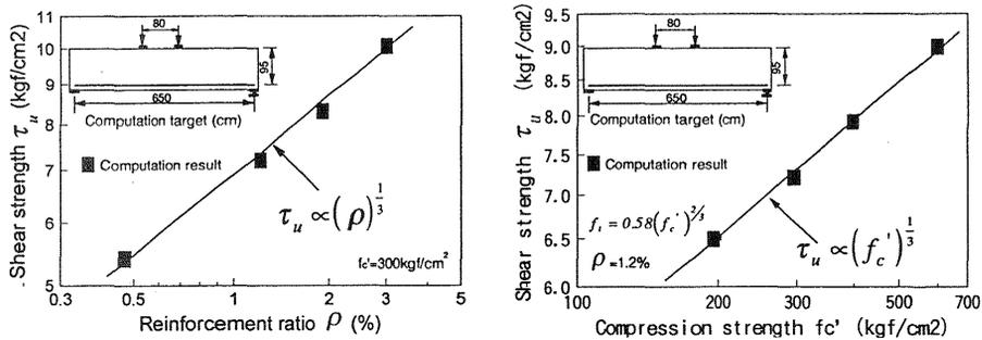
Fig. 5. FEM computational results compared with JSCE code
