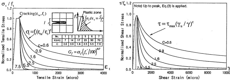
Fig. 3. Tension and shear strain softening model for concrete in PL zone
