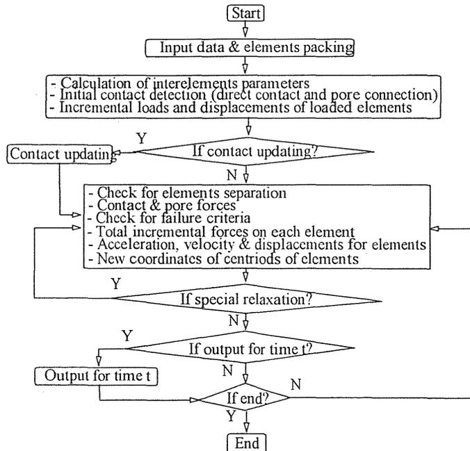
Fig. 2. Flow of fracture analysis and failure monitoring with DEM
