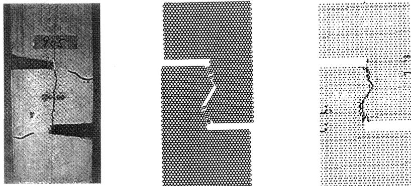
(a) General failure mode (test) (b) Failure mode (analysis) (c) Crack pattern (analysis)
