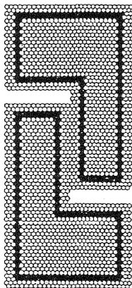
Fig. 4. The DEM model for one-plane shear test used in analysis
