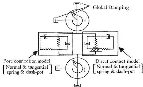
Fig. 1. Contact and pore medium models
