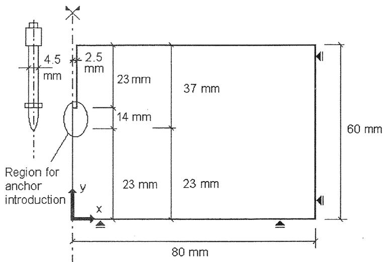
Fig. 4. Geometry of the specimen for testing of powder actuated anchors
