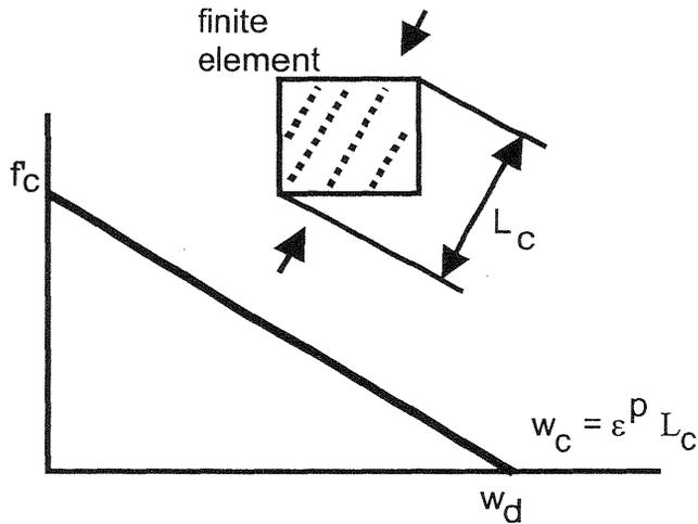
Fig. 2. Compressive softening and compressive characteristic length.
