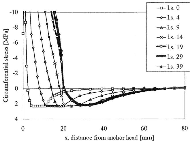
Fig. 6. Evolution of circumferential stresses around the anchor head showing the radial crack closure. Load step 19 is the end of insertion and load step 29 is at the peak pull-out force.
