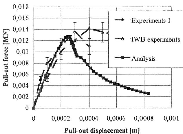
Fig. 5. Comparison of the finite element analysis with experimental data.
