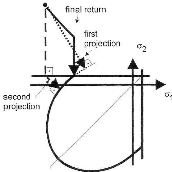
Fig. 3. Schematic description of the iterative process (16). For clarity shown in two dimensions.
