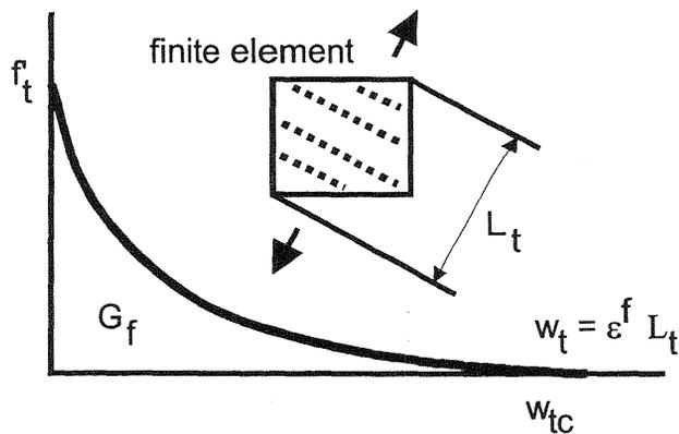
Fig. 1. Tensile softening and characteristic length
