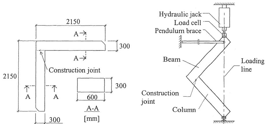
Fig. 2. Dimensions of specimens and test set-up.
