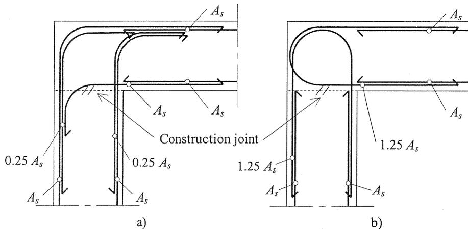
Fig. 1. Detailing of the reinforcement according to: a) the conventional method, and b) the new alternative.  $A_s$  denotes the reinforcement area.
