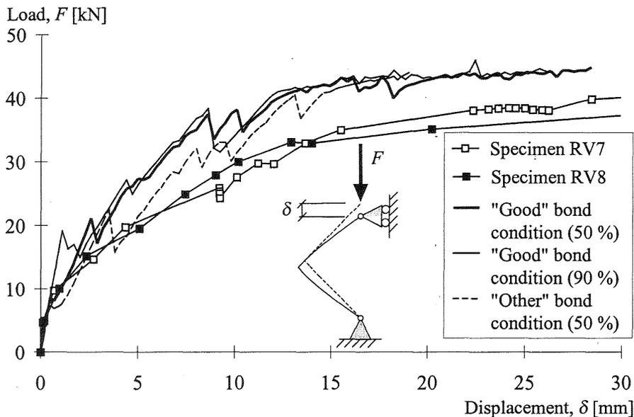
Fig. 5. Load-displacement relations for the tests and FE analyses with the new reinforcement detailing. Values between brackets show the strength of the concrete modelling the construction joint.
