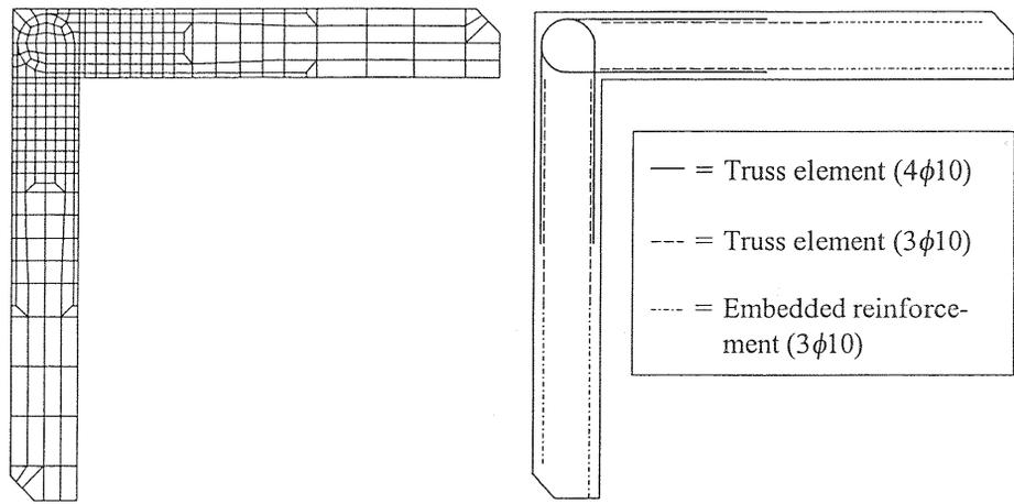
Fig. 4. The finite element mesh and modelling of the reinforcement bars of the frame corner with new reinforcement detailing.
