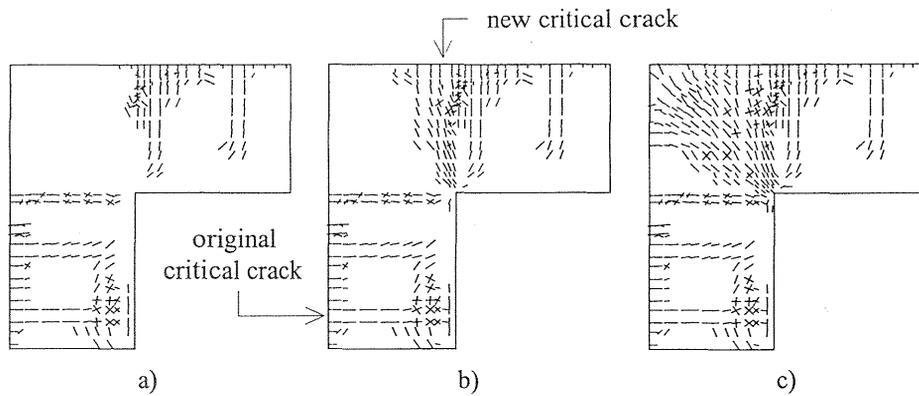
Fig. 7. Crack propagation in the corner area for the conventional reinforcement detailing at the load levels marked in Fig. 6.
