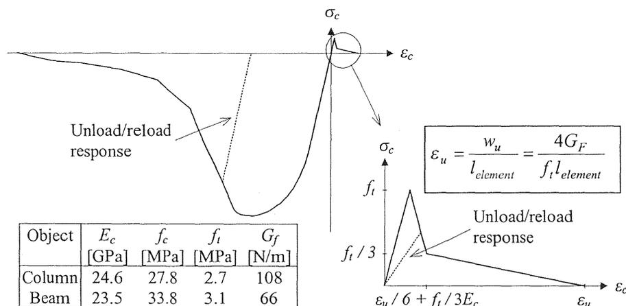
Fig. 3. Stiffness used in the analyses for unloaded concrete in compression and tension ( $l_{element} = s_{rm}/2$  when perfect bond is assumed).
