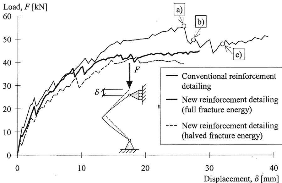
Fig. 6. Comparison of the load-displacement relations for frame corners carried out with new and with conventional reinforcement detailing.
