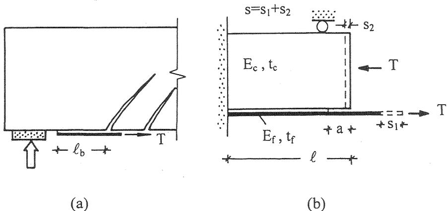
Fig. 2. (a) FRP plate anchorage zone; (b) simple model for describing bond failure in the anchorage zone.
