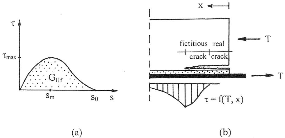
Fig. 3. (a) Local bond constitutive law according to NLFM; (b) fictitious crack model for bond failure in the anchorage zone.
