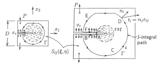
Fig. 1 Path of J-integral for size effect analysis
