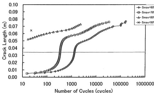
Figure 7. Fatigue crack growth in a beam overlaid with 3 % FRC (beam height = 0.1 m and FRC thickness ratio = 0.66).
