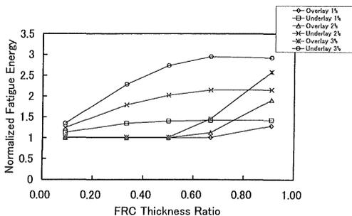
Figure 10. Normalized fatigue energy for beam height = 0.1 m.
