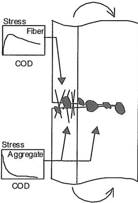
Figure 1. FRC underlaid beam under monotonic loading.
