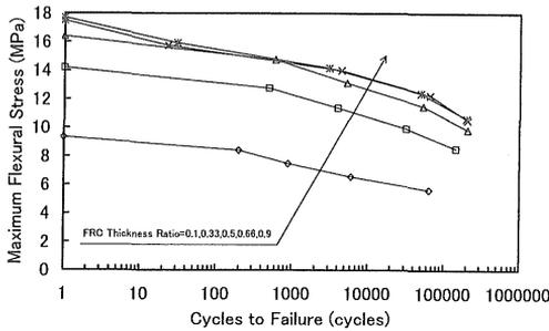
Figure 9. Fatigue life of underlaid beams with varied FRC thickness ratio for beam height = 0.1 m.  $V_f = 3\%$  only.
