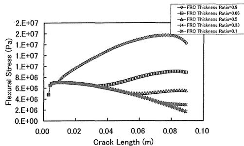
Figure 3. Crack propagation in a beam overlaid with 3 % FRC for varied FRC thickness ratios.
