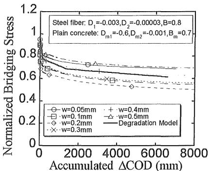
Figure 2. Crack bridging degradation with different initial opening displacements,  $w$ .
