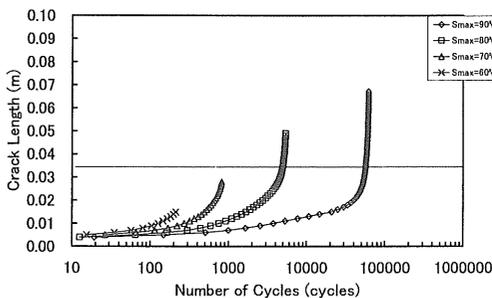
Figure 5. Fatigue crack growth in a beam overlaid with 1 % FRC (beam height = 0.1 m and FRC thickness ratio = 0.66).
