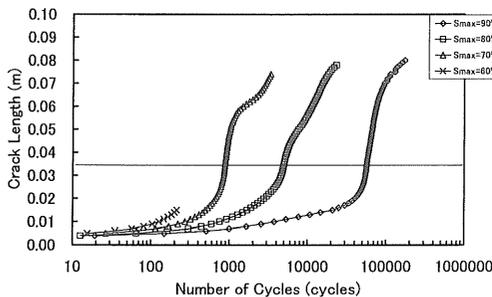
Figure 6. Fatigue crack growth in a beam overlaid with 2 % FRC (beam height = 0.1 m and FRC thickness ratio = 0.66).
