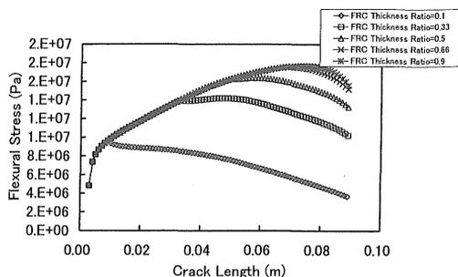
Figure 4. Crack propagation in a beam underlaid with 3 % FRC for varied FRC thickness ratios.
