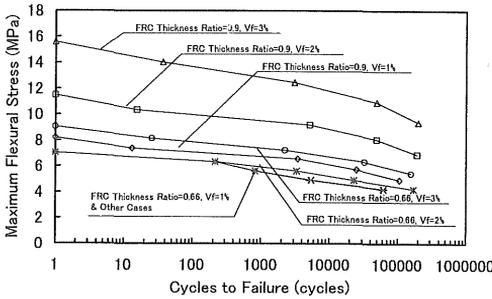
Figure 8. Fatigue life of overlaid beams with varied FRC thickness ratio for beam height = 0.1 m.
