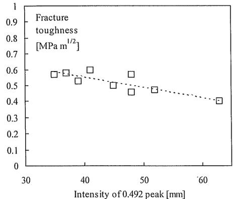
Figure 6. Fracture toughness  $K_{Ic}$  vs. amount of portlandite.
