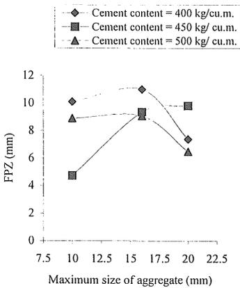
Fig. 2: Variation of FPZ with maximum size of coarse aggregate.
