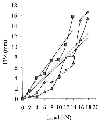
Fig. 1: Typical diagram showing the variation of FPZ with load in HSC.
