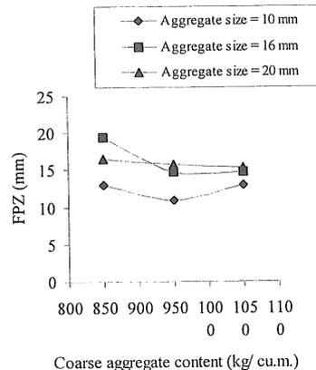
Fig. 4: Variation of FPZ with coarse aggregate content.
