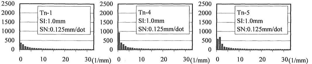
Figure 8(b) Results of FFT One-dimensional analyses of the tensile crack surface on the measurement crack line (y-axis direction)
