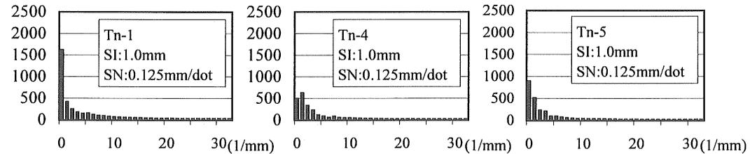
Figure 7(a) Result of FFT one-dimensional analysis of the tensile crack surface on the measurement reference plane (x-axis direction)
