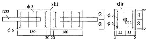
Figure 3 Concrete specimen used in the tensile experiment
