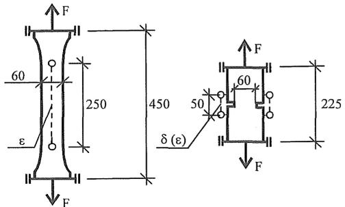
Figure 1. Geometrical dimensions of the investigated specimens (thickness of both specimens  $d = 100$ ; data in [mm]).
