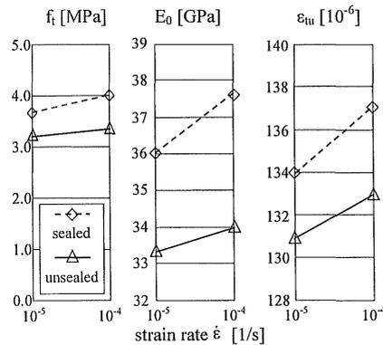
Figure 3. Effect of the strain rate and the curing conditions on the uniaxial tensile strength (left), the Young's Modulus (middle) and the elongation at failure (right).
