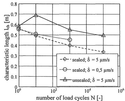
Figure 7. Effect of the number of load cycles to failure on the characteristic length for different deformation rates and curing conditions.
