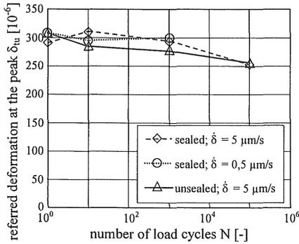
Figure 5. Effect of the number of load cycles to failure on the deformation at the peak stress for different deformation rates and curing conditions.
