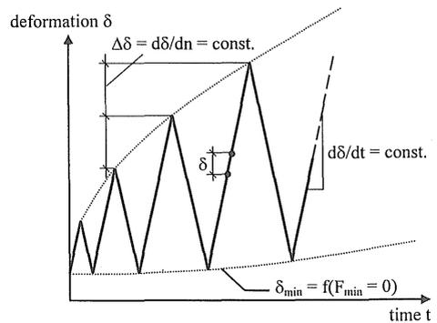
Figure 2. Test control in the fatigue experiments.
