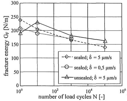
Figure 6. Effect of the number of load cycles to failure on the fracture energy for different deformation rates and curing conditions.
