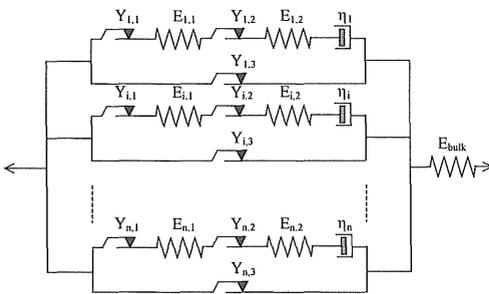
Figure 9. Rheological statistical model for the description of the fatigue behaviour of concrete under tensile loading conditions.
