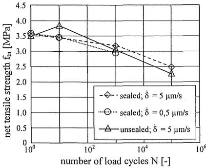
Figure 4. Effect of the number of load cycles to failure on the net tensile strength for different deformation rates and curing conditions.
