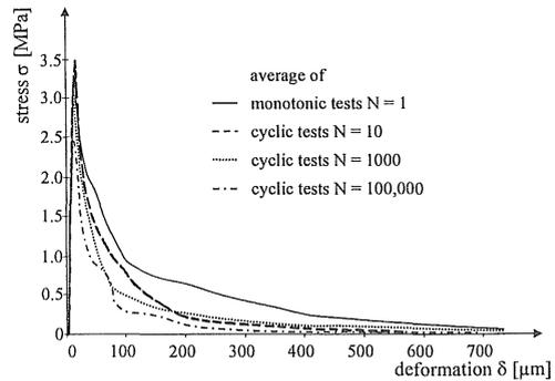
Figure 8. Envelope curves of the stress-deformation relations obtained from the monotonic and the fatigue tests performed on sealed specimens.
