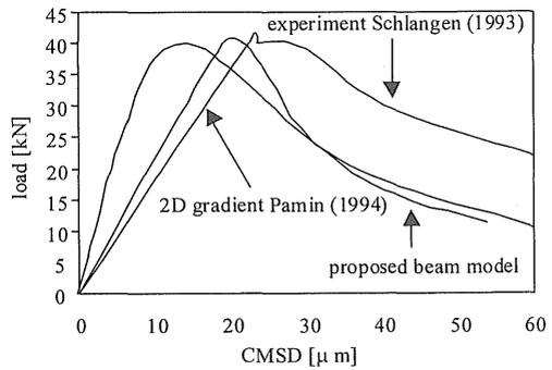
Figure 4. Load versus Crack Mouth Sliding Displacement [CMSD] of the four-point-shear test
