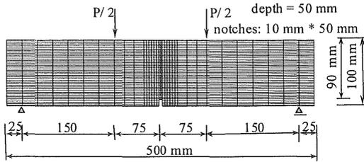
Figure 1. Geometry of the notched beam
