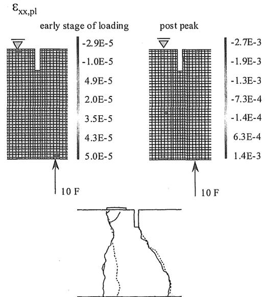
Figure 5. Crack pattern of the shear test a) beam model, b) experiment (Schlangen 1993)
