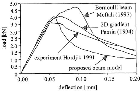
Figure 2. Load deflection diagram of the four-point-bending test
