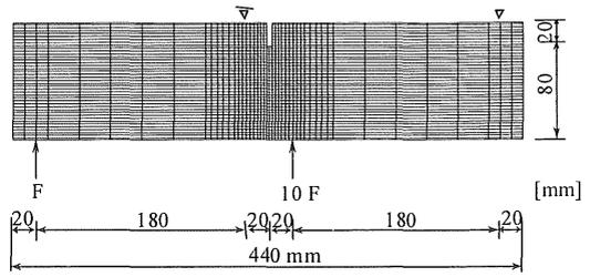
Figure 3. Geometry of the four-point-shear test beam
