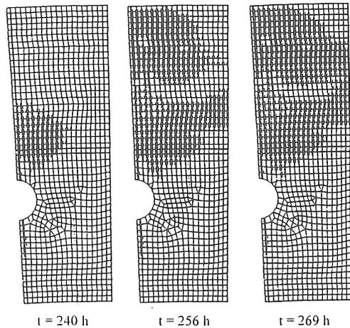
Figure 11. Development of cracks during the first pressure and temperature increase
