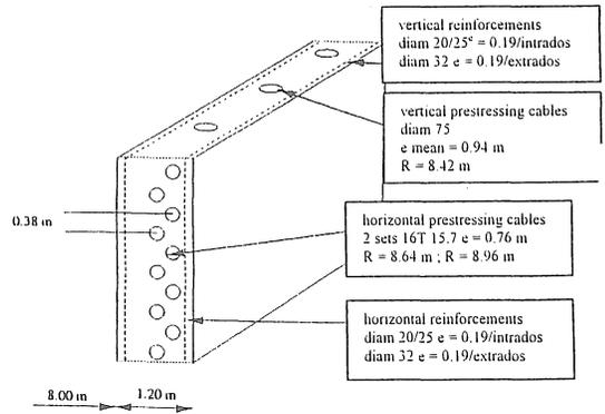
Figure 3. Layout of the prestressing cables and reinforcements
