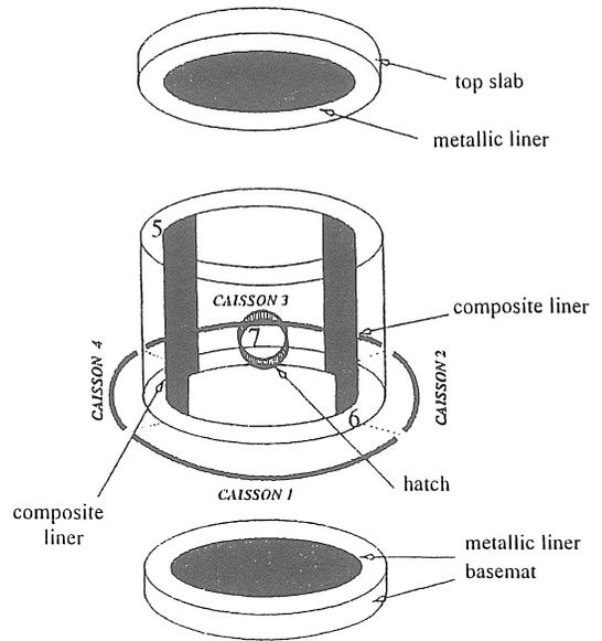
Figure 2. Principle of the leaks measurements
