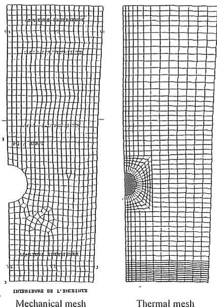
Figure 7. Meshes used for the model
