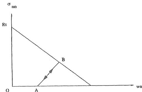
Figure 8. Concrete behaviour along the normal to a crack
