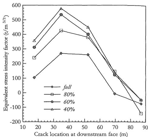
Figure 6. Equivalent stress intensity factor at downstream face according to reservoir water level variation
