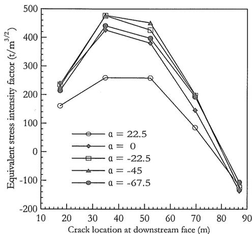
Figure 4. Equivalent stress intensity factors at the downstream face according to crack locations and directions (Air temperature = -10 °C)
