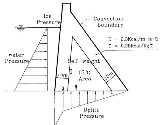
Figure 3. Applied loads and thermodynamic properties for thermal transfer analysis
