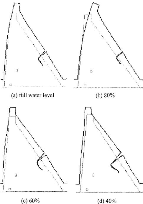
Figure 7. Configurations of crack propagation according to reservoir water level (crack D,  $\alpha=0^\circ$ )
