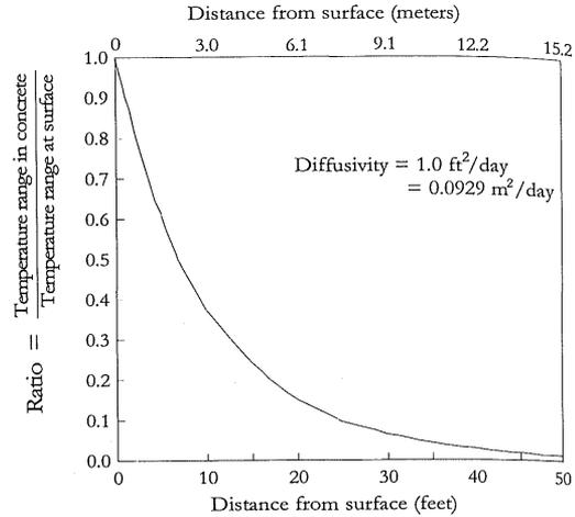
Figure 2. Ratio of temperature variation with depth
