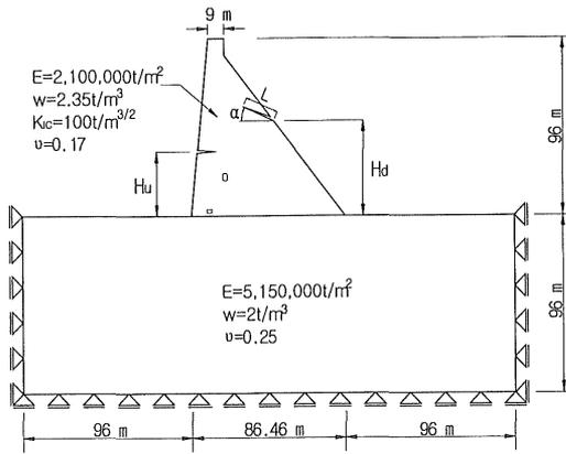
Figure 1. Dam cross section and boundary condition
