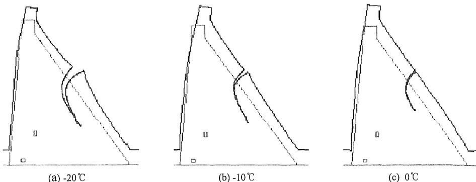
Figure 5. Configurations of crack propagation according to variation of air temperatures (crack C,  $\alpha=45^\circ$ )
