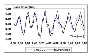
Figure 17. High -Level pseudodynamic test: Time history of the base shear.
