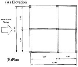
Figure 2. Layout of the specimen; (A) Elevation, (B) Plan
