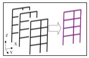
Figure 7. Equivalent RC frame.
