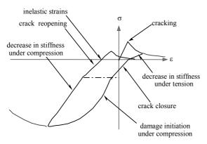
Figure 5. Uniaxial damage model for concrete.
