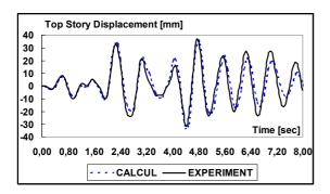
Figure 12. Low-Level pseudodynamic test: top displacement versus time.
