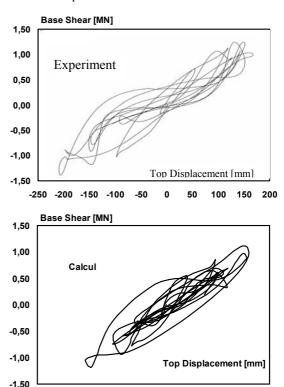
Figure 18. High-Level pseudodynamic test: base-shear versus top-story displacement diagram.
