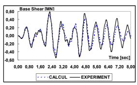
Figure 13. Low-Level pseudodynamic test: base shear versus time.
