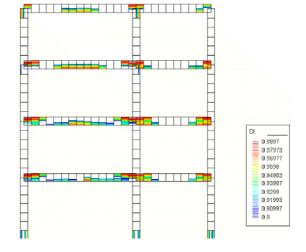
Figure 15. Damage pattern at the end of the Low-Level pseudodynamic test.
