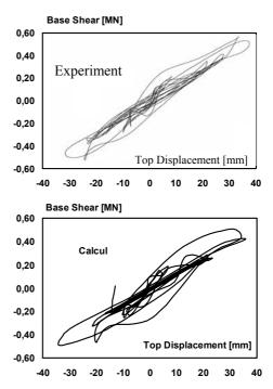
Figure 14. Low-Level Level pseudodynamic test: base-shear versus top-story displacement diagrams.
