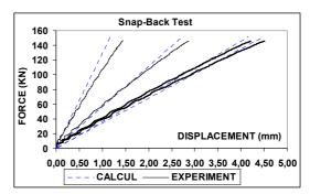
Figure 10. Simulation of the first Snap-Back test (loading applied at the third story).
