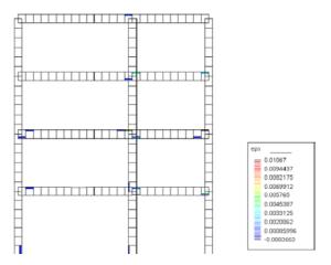
Figure 19. Position of yielded reinforcement bars at the end of the High-Level pseudodynamic test.
