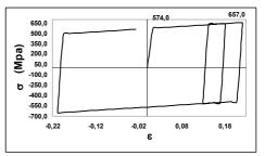
Figure 6. Uniaxial plasticity law for reinforcement bars.
