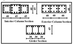
Figure 8. Section of columns and beams of the equivalent RC frame.
