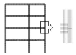
Figure 9. Mesh of the structure with multi-layer beams
