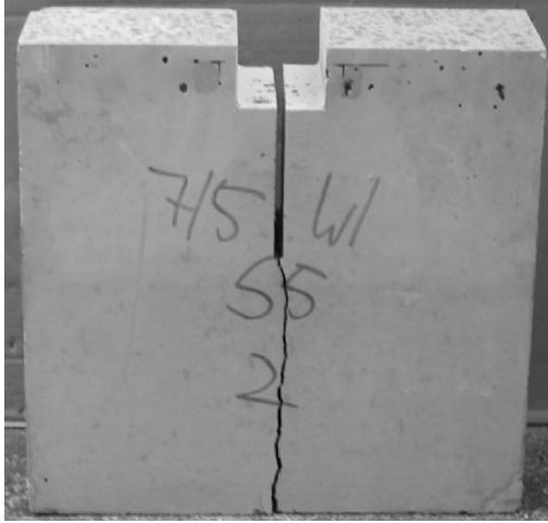
Figure 7. Crack formation in wedge splitting specimen
