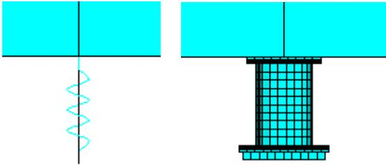
Figure 7. Non-linear spring and 3D model of a steel support
