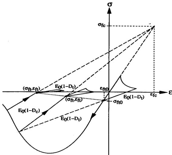
Figure 8. PRM modeling of the concrete behavior
