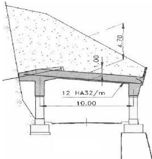
Figure 1. Schematic view of a conventional rock shed
