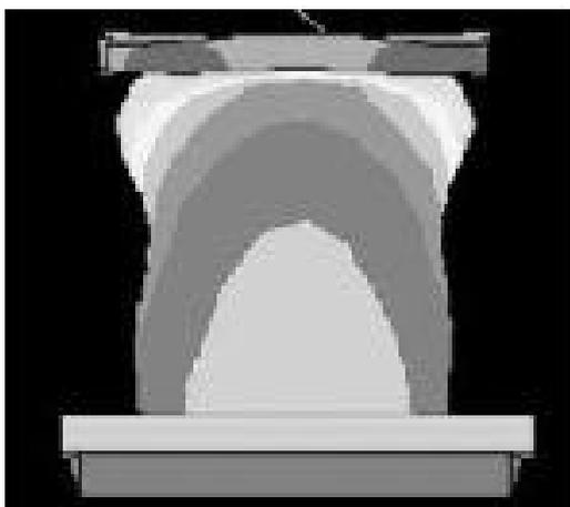
Figure 12. Deformed shape of the experimental and modeled steel support
