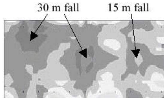
Figure 14. Damage pattern due to tension ( $D$ , eq. (5)) on the sub-face of the slab. The darker the slab, the more damaged it is.
