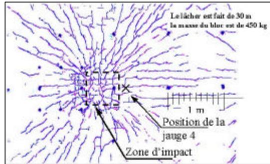
Figure 13. Mapping of damage distribution in the slab
