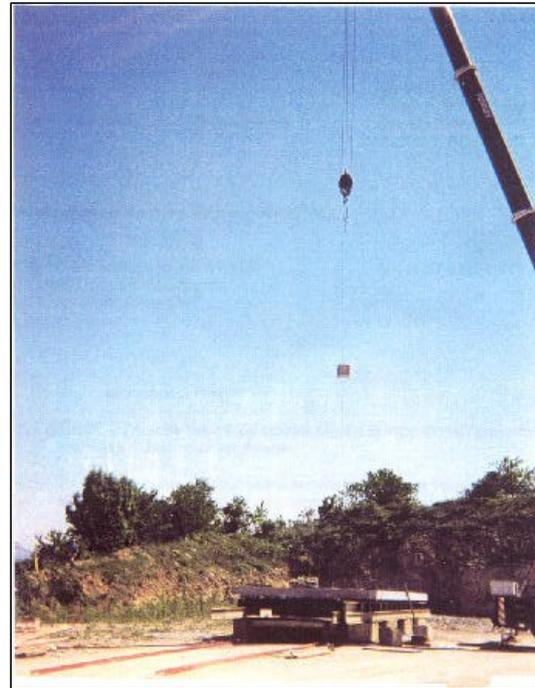
Figure 5. Rock fall test
