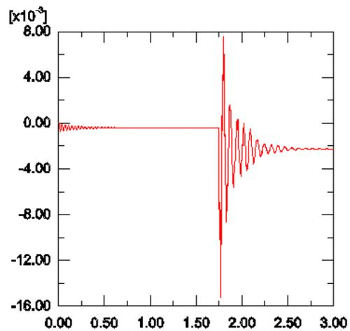
Figure 11. Displacement of the bottom face of the slab at the location of impact versus time
