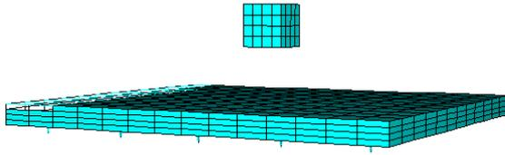
Figure 6. Three dimensional modeling of the slab and the block
