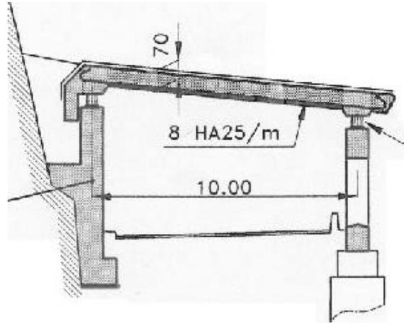
Figure 2. Schematic view of the new rock shed system
