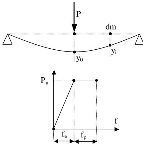
Figure 4. Simplified model used for the design of the concrete slab
