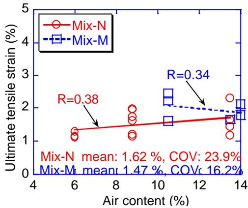
Figure 11. Effects of air content on the ultimate tensile strain (TP test).
