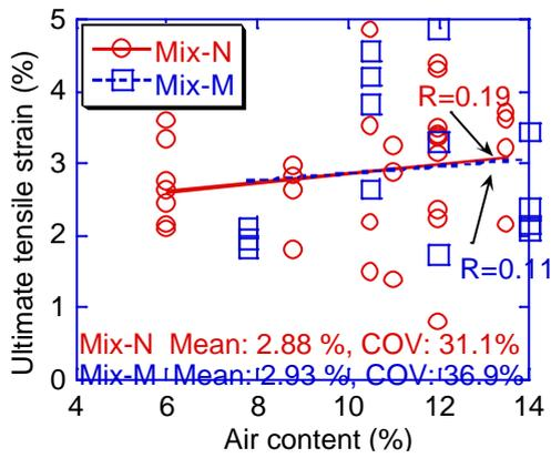
Figure 9. Effects of air content on the ultimate tensile strain (TC test).
