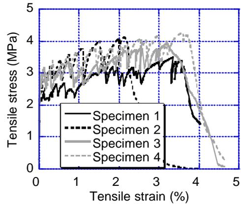
Figure 5 Stress-strain curves under tension – TC test (N6)
