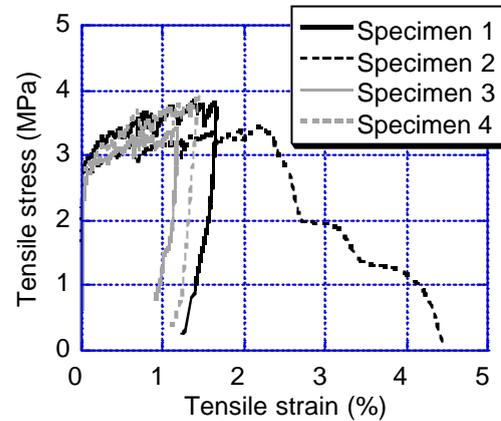
Figure 6. Stress-strain curves under tension – TP test (N6)
