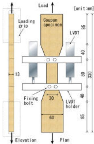
Figure 1. Tensile test of plate shaped specimen (TC test).
