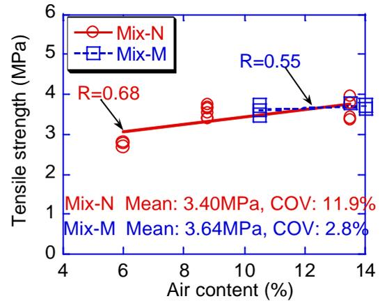
Figure 12. Effects of air content on tensile strength (TP test).
