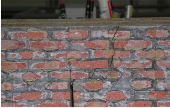
Figure 6. Crack in a large size TPB specimen with the bed joints at  $0^\circ$  after testing.
