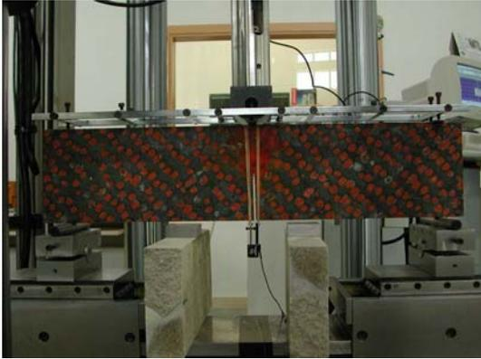
Figure 1. Testing arrangement to measure the fracture properties of the brick masonry (bed joints at 45°).
