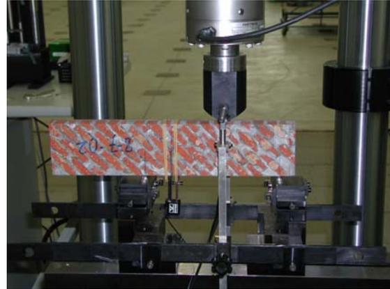
Figure 4. TPB small specimen ( $D = 75$ mm), with the bed joints inclined  $-45^\circ$ , during testing.
