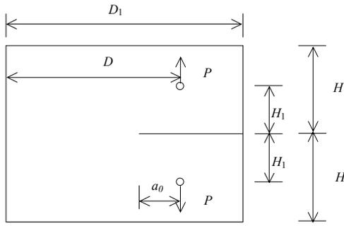
Fig.5 The configuration of the compact tension specimen
