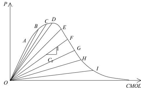
Fig. 1 The sketch of linear asymptotic superposition of  $P$ - $CMOD$  curve
