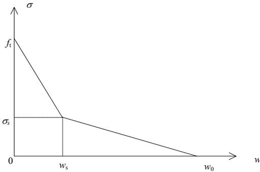
Fig.2 A bilinear softening traction-separation curve
