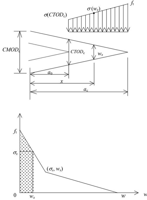
Fig.3 The distribution of cohesive force along the FPZ for  $CTOD_c \leq w_s$
