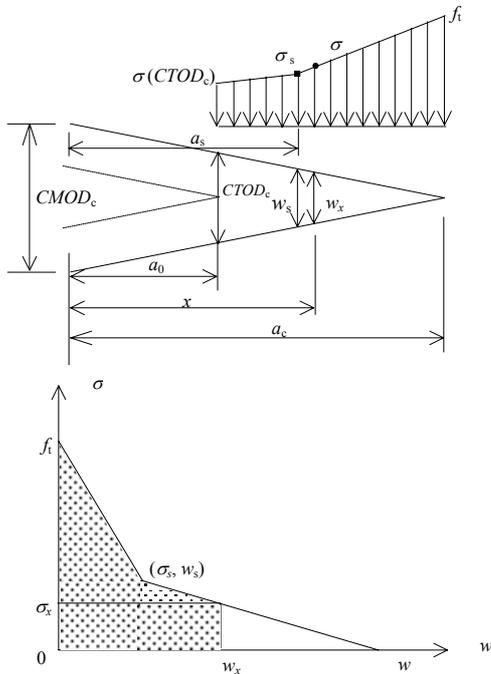
Fig.4 The distribution of cohesive force along the FPZ for  $w_s \leq CTOD_c \leq w_0$
