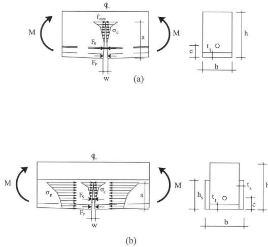
Figure 6. Free body diagram of the dominant flexural crack in retrofitted beams. Beams retrofitted with (a) one tension strip, and (b) one tension and two side strips.
