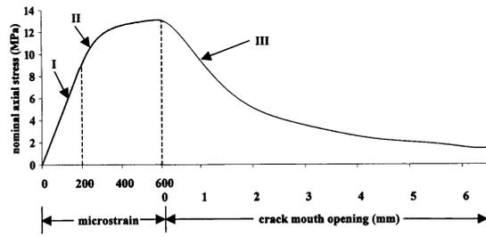
Figure 2. Complete pre- and post-peak tensile curve for CARDIFRC® as prescribed by Equations (1) to (3).
