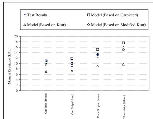
Figure 7. Comparison of the moment resistance of the stage II beams with the predictions of the second model.
