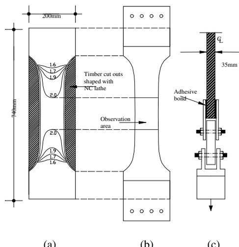
Figure 1. Special tensile specimen geometry, showing (a) contours of tensile stress under a unit external tension, (b) the observation area with a uniform and well-defined tension field and (c) the load application arrangement.
