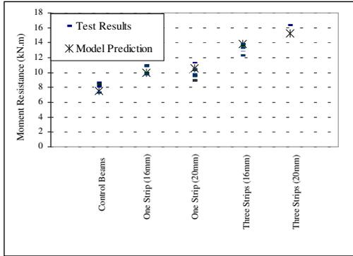
Figure 4. Comparison of the moment resistance of the stage I beams with the predictions of the first analytical model.
