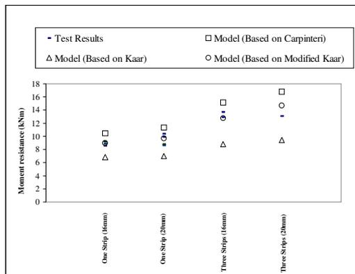
Figure 8. Comparison of the moment resistance of the stage I beams with the predictions of the second model.
