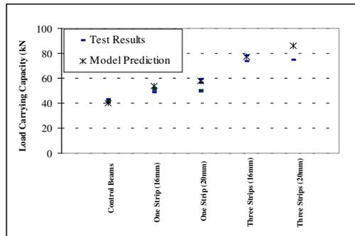
Figure 5. Comparison of the load carrying capacity of the stage II beams with that predicted by the first analytical model.
