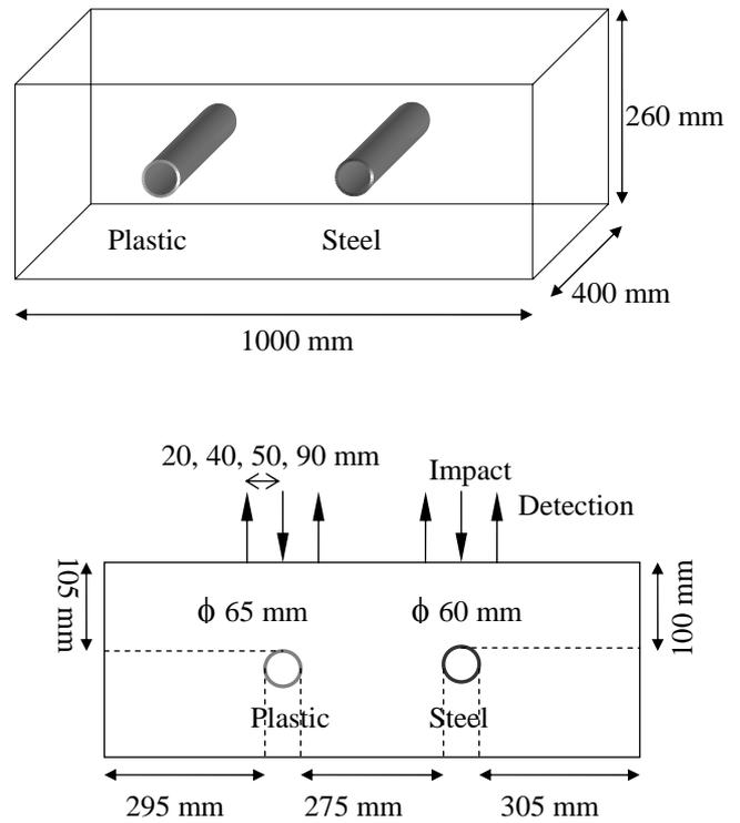
Figure 2. Concrete specimen tested.
