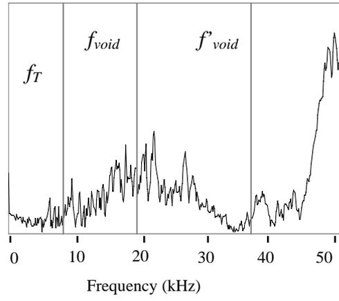
b) Left accelerometer above plastic sheath
