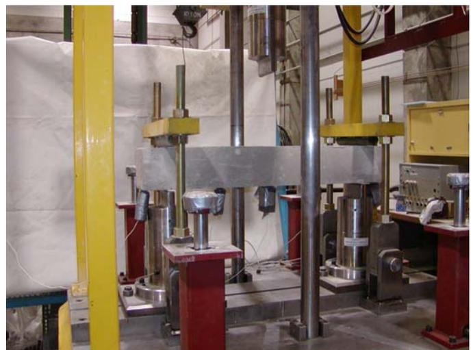
Figure 1. Impact test setup with steel yokes.
