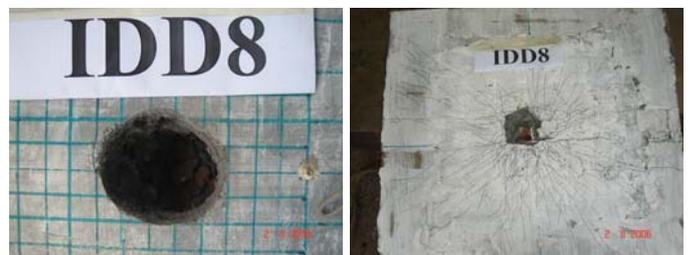
Figure 19. Impact and distal face of IDD8 after perforation.
