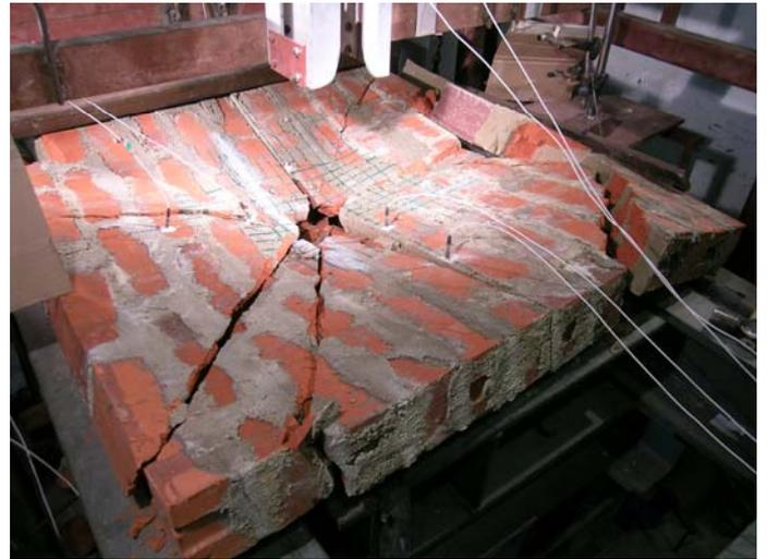
Figure 9. Failure of unreinforced masonry wall under impact loading.
