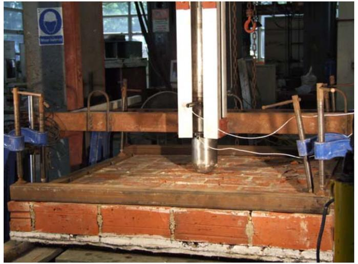
Figure 5. Low-velocity projectile impact load test set-up.
