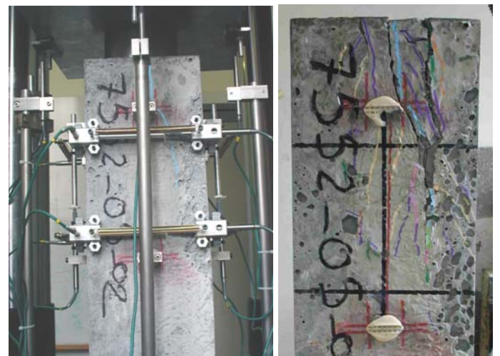
Figure 3. Crack pattern evolution. Block 1 side D. (left) at first cracking - (right) after failure.
