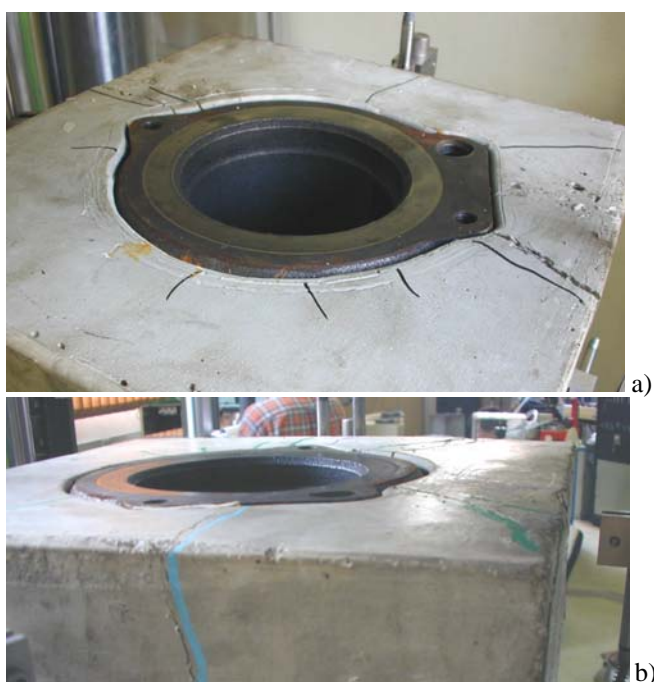
Figure 13. Punching of the steel anchor plate. a) Block 10 after failure. b) Block 11 after failure.
