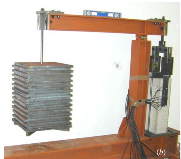
Figure 1. (a) Geometry of specimens and (b) experimental setup for long – term tests.
