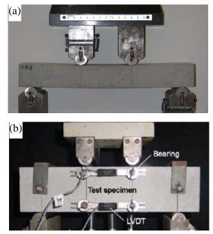
Figure 4. Comparison of test setup for the (a) UM method and (b) JCI method.
