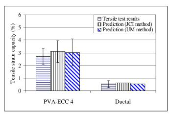
Figure 6. Comparison of tensile strain capacity from UTT with predictions from JCI method and proposed UM method for different SHCCs. (Experimental data for both UTT and FPBT are from JCI round robin test and only two FPBT specimens were reported for Ductal.)
