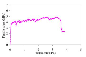
Figure 1. Typical tensile stress-strain curve of ECC.
