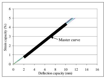
Figure 3. Tensile strain capacity –deflection capacity relation obtained from parametric study (20 cases) and simplified master curve (with uniform thickness).
