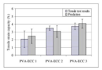
Figure 5. Comparison of tensile strain capacity from UTT test with prediction from proposed UM method for different PVA-ECCs.
