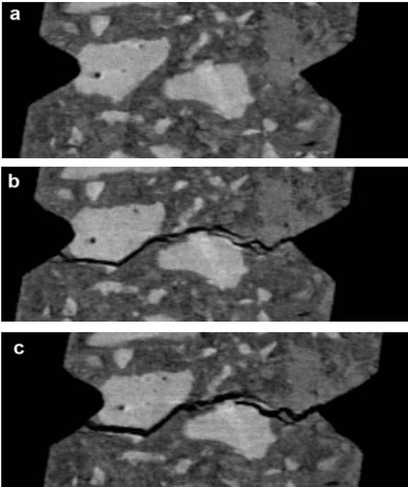
Figure 3a-c. 2D crack reconstructions, displacement vector fields and crack bridging: (a-c) 2D vertical slices from 3D SR $\mu$ CT reconstruction of the notched area of the same specimen for three subsequent loading stages ('A', 'B' and 'C').
