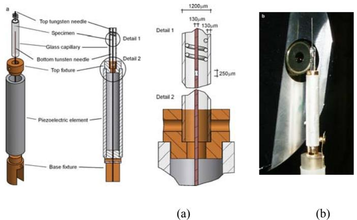
Figure 2. In-situ SR $\mu$ CT microtensile testing device: (a) Schematic view of the microtensile device based on piezoelectric actuation, and (b) Photograph of the device in front of the SR $\mu$ CT detector
