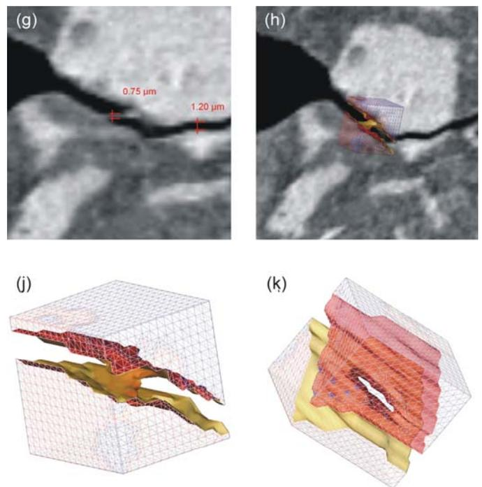
Figure 3g-k. Detail of one of the vertical slices showing one of the bridging events with the sizes of the bridge and crack in micrometers; (h-k) 3D reconstruction of the bridge shown in Figure 3g
