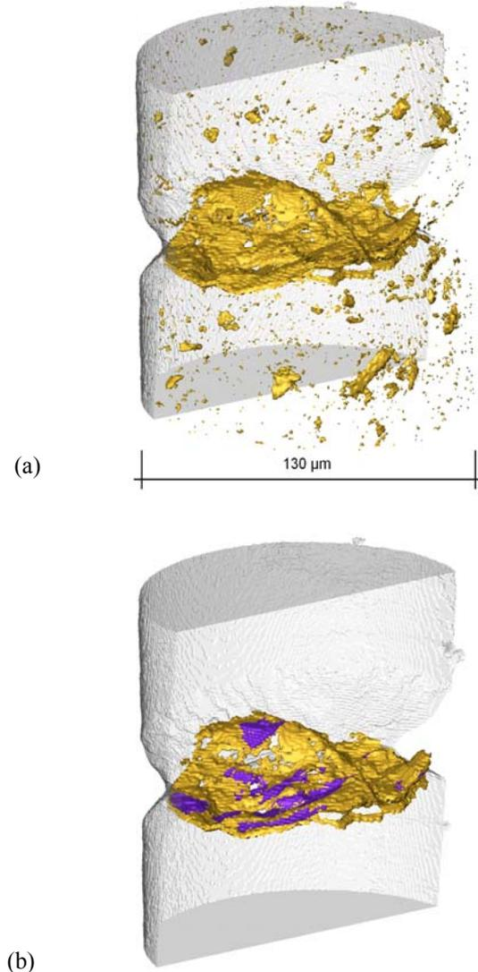
Figure 4. 3D reconstruction of crack with respect to cement microstructure: (a) 3D reconstruction of the crack surface area and porosity in the microspecimen in the stage 'B' shown in 2D in Figure 3b; (b) 3D reconstruction of the major tensile crack in the microspecimen in the stage 'B' showing the areas (dark purple colour) in which the crack intersects the unhydrated cement particles.
