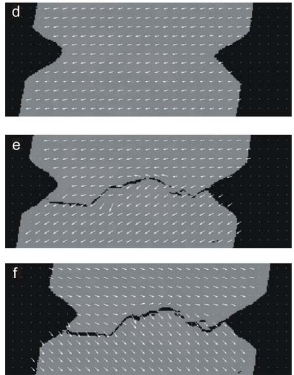
Figure 3d-f. Vector fields showing the displacement between the respective loading stage ('A', 'B' or 'C') and the unloaded state of the specimen.
