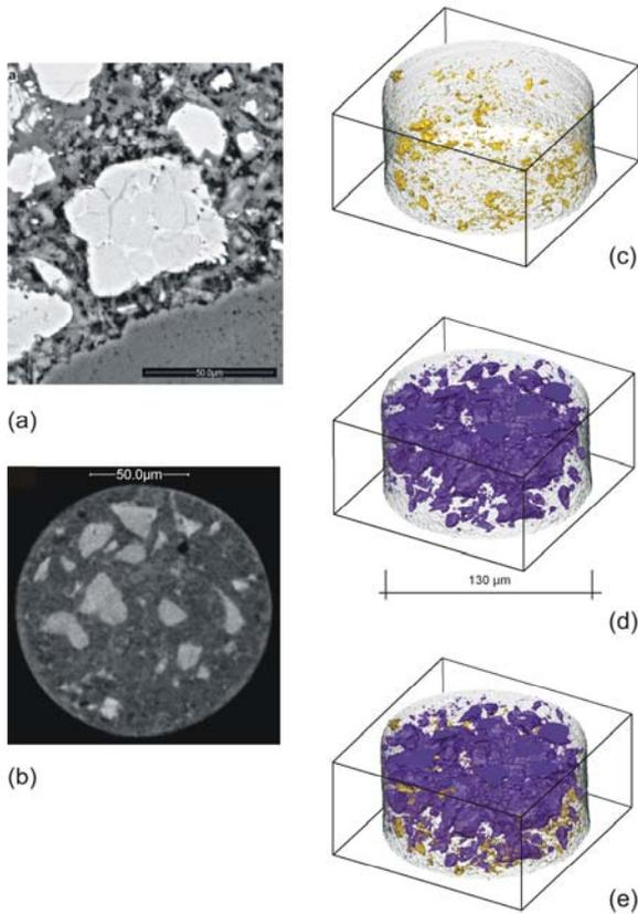
Figure 1. Comparison of ESEM and SR $\mu$ CT: (a) Micrograph of the polished surface of hydrated Portland cement. (b) Axial slice from 3D SR $\mu$ CT reconstruction of a cylindrical specimen of hydrated Portland cement. 3D-reconstruction of voids (c), unhydrated cement grains (d), and the relationship between the two (e) in part of the volume of 130 $\mu$ m-diameter specimen.
